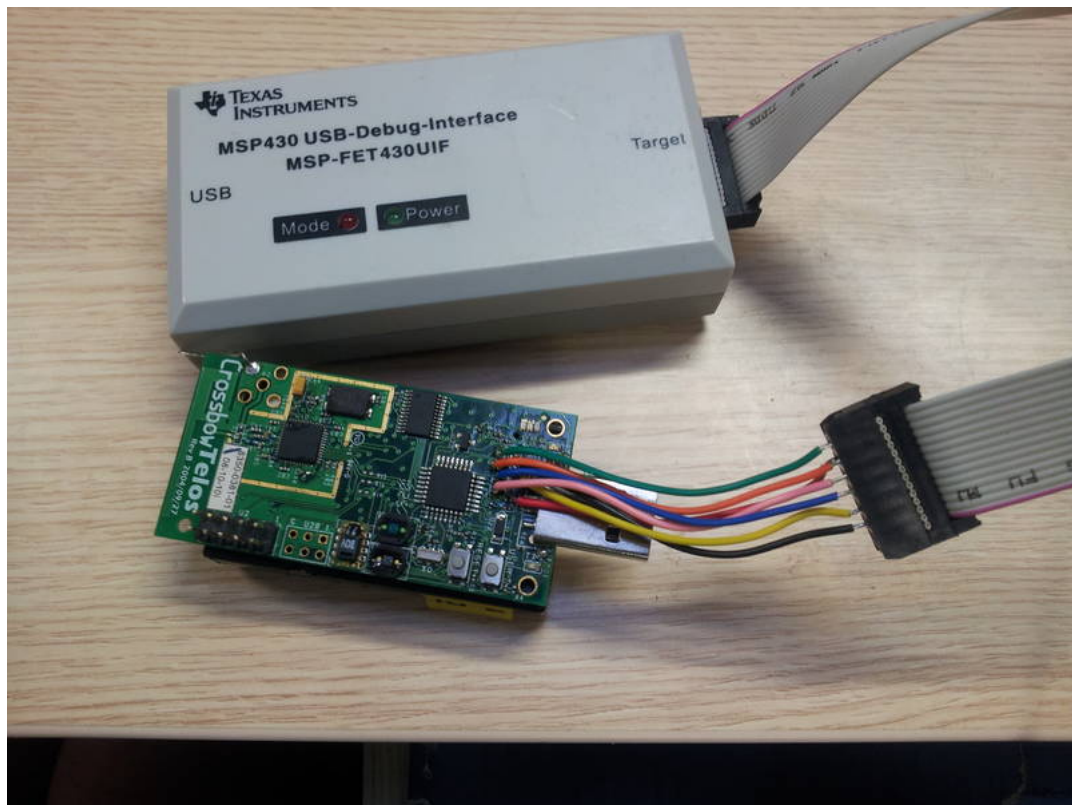
Figure 6.1: TelosB hardware connected to the MSP-FET430 USB debugger
