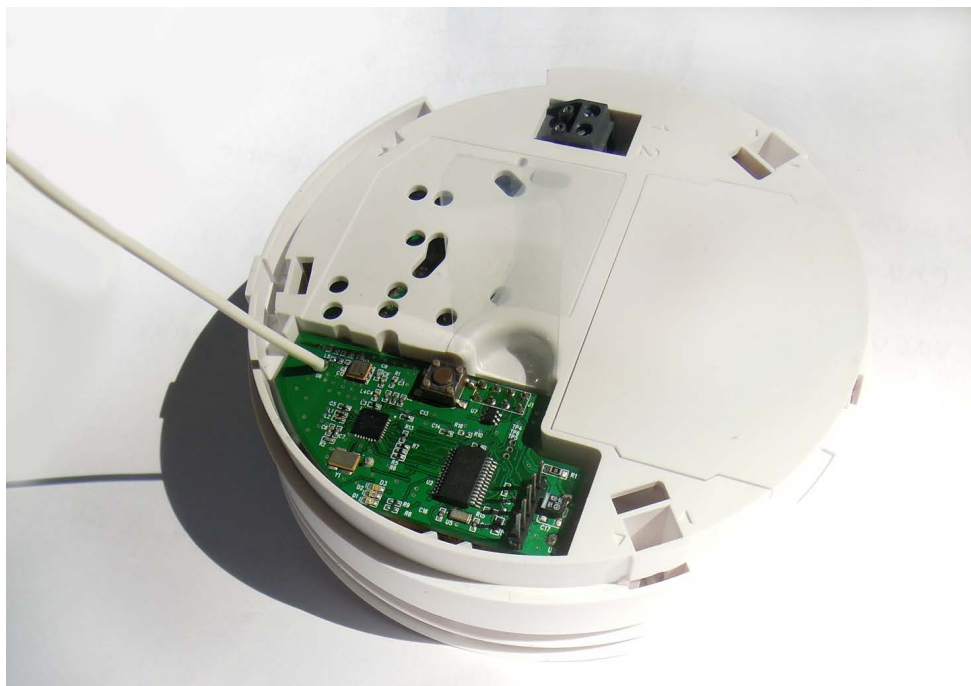
Figure 2.9: FireMote in Alarm Housing
