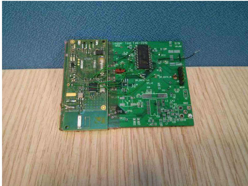
Figure 2.3: Prototype of SX1211 and PIC24F
