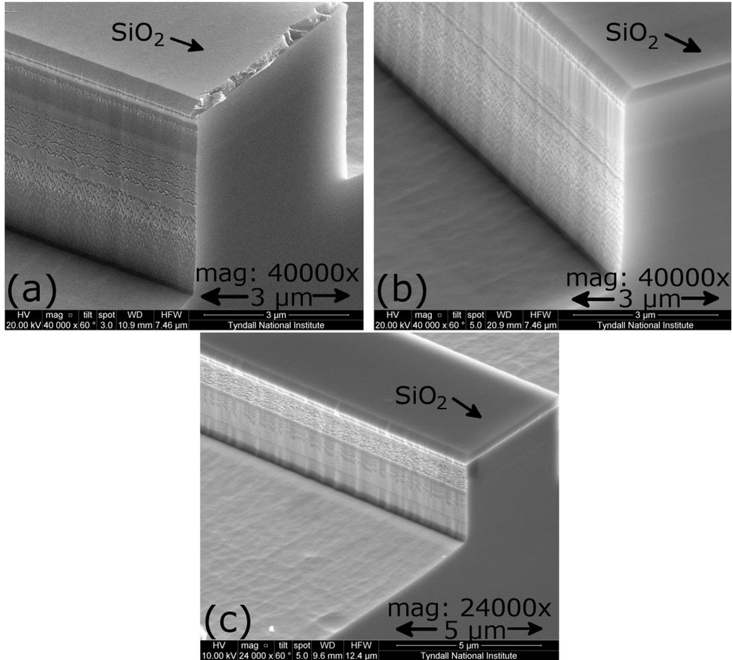
**Figure 9.19:** Cross-section sidewall SEM images, (a)  $\text{Cl}_2/\text{CH}_4/\text{H}_2 = 10/15/20$  sccm sidewall roughness value 3, (b)  $\text{Cl}_2/\text{CH}_4/\text{H}_2 = 4/7/20$  sccm sidewall roughness value 5, (c)  $\text{Cl}_2/\text{CH}_4/\text{H}_2 = 4/15/10$  sccm sidewall roughness value 7
