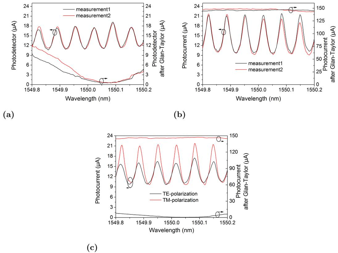
**Figure 6.10:** Fabry-Pérot spectrum (1550 nm) of Filter1 (cavity length: 5400 μm) and the polarization state of the TLS beam (a) for the TE-polarization, (b) and the TM-polarization, (c) comparison of both polarizations.
