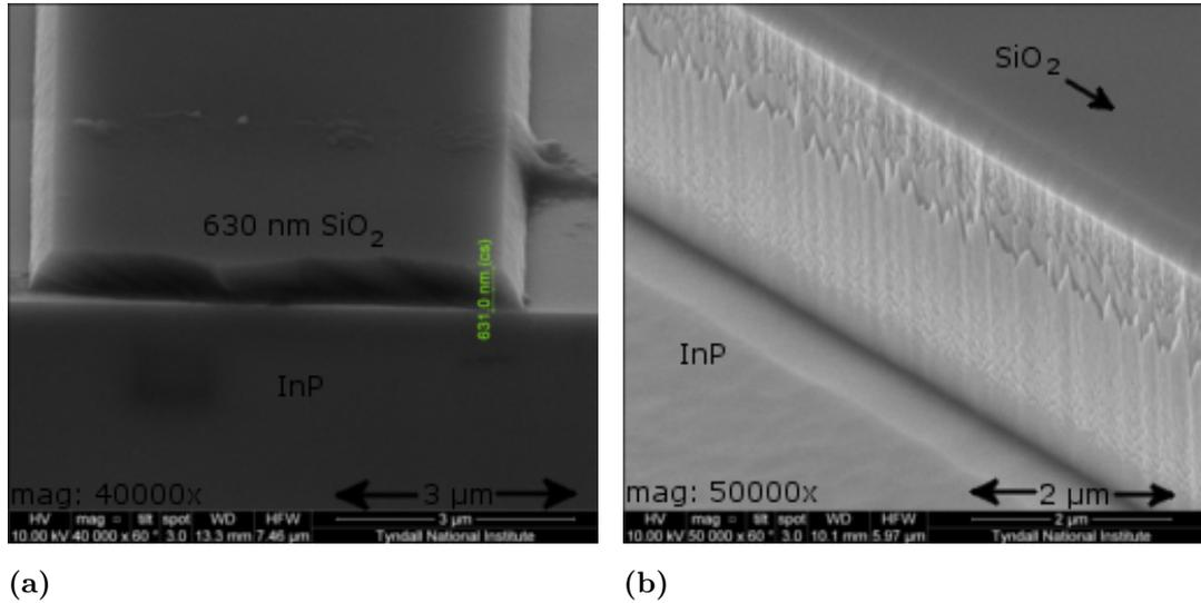
**Figure 9.14:** Cross-section SEM images of  $\text{SiO}_2$  on  $\text{InP}$ . (a) before the  $\text{InP}$  etch, (b) after the  $\text{InP}$  etch.
