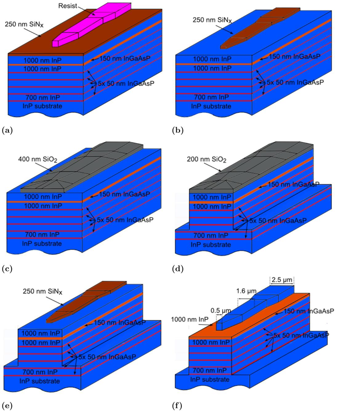
**Figure 9.1:** Consecutive process steps used, (a) after the first lithography step, (b) after the  $\text{SiN}_x$  mask is patterned, (c) after the  $\text{SiO}_2$  layer is patterned, (d) after the first 4  $\mu\text{m}$  deep III-V material ICP etch, (e) after the overlying  $\text{SiO}_2$  mask is removed by wet chemical etching, (f) the final ATG structure with the  $\text{SiN}_x$  mask removed.
