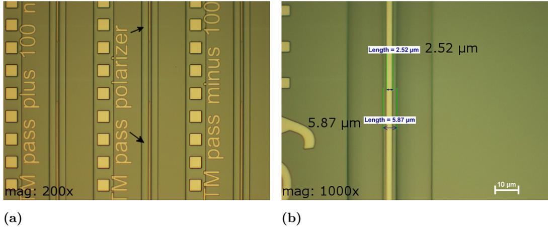
**Figure 9.39:** Microscope images after the ICP removal of the second  $\text{SiO}_2$  mask. (a) Section with two TM-pass polarizers, (b) unmodified ATG along the whole section.
