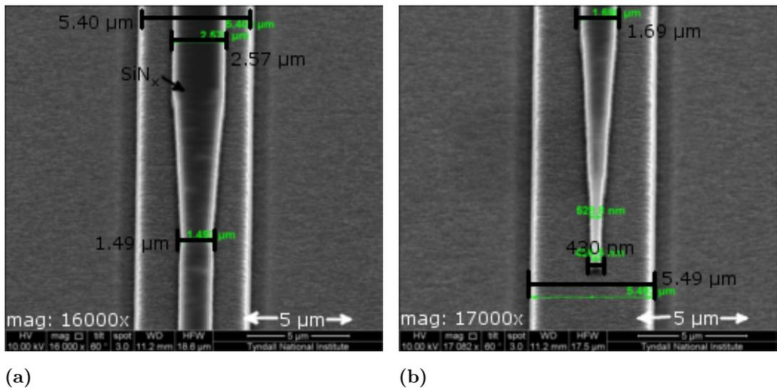
**Figure 9.10:** SEM images of a resonant coupler 200 nm wider than ideal after a 7 min 45 s and 2 min 45 s  $\text{Cl}_2/\text{N}_2$  etch. (a) top view of the taper to the mode beating section, (b) top view of the end taper.
