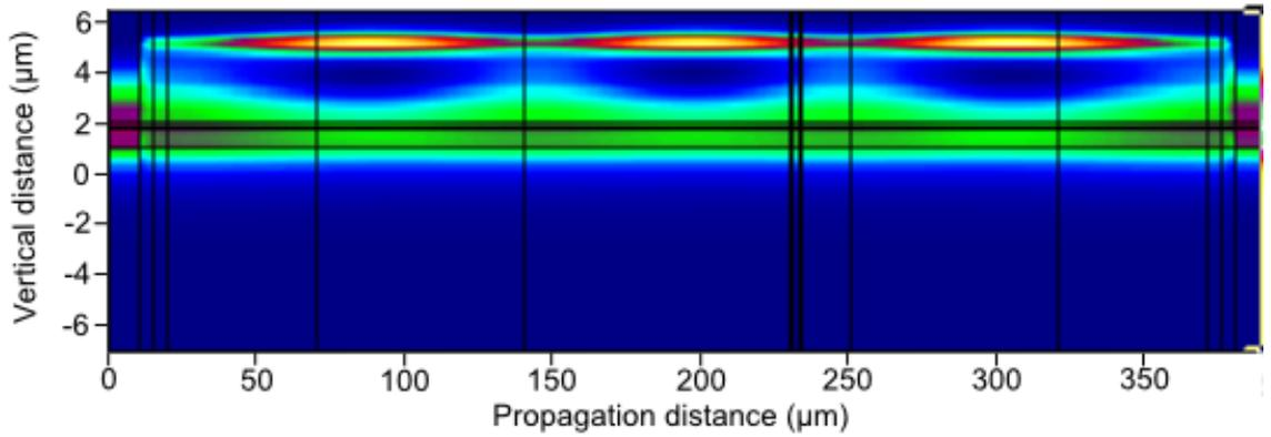
**Figure 6.4:** Side view of the intensity distribution of the TE-field, the input is on the left side in the lower waveguide. The vertical lines correspond to section boundaries.
