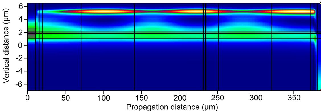
**Figure 6.2:** Side view of the intensity distribution of the TE-field, the input is on the left side in the lower waveguide. The vertical lines correspond to section boundaries.
