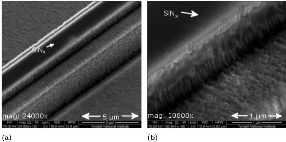
**Figure 9.12:** Cross-section SEM images of a constant ATG after a 7 min 45 s and 2 min 45 s  $\text{Cl}_2/\text{N}_2$  etch. (a) sidewall of the upper and lower waveguide, (b) sidewall of the upper waveguide.
