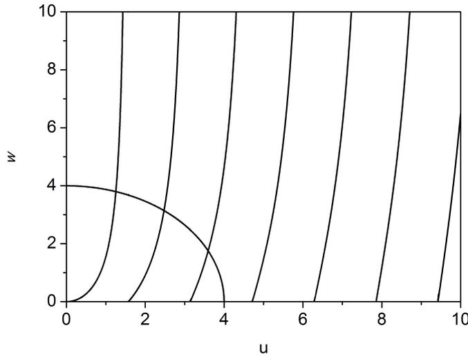
**Figure 2.2:**  $u - w$  relationship in a symmetric slab waveguide.
