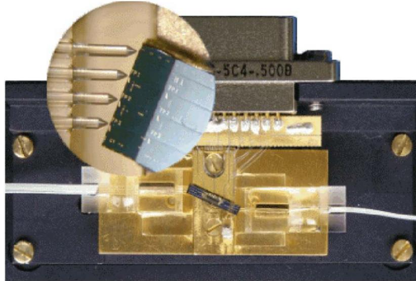
**Figure 1.3:** *Photograph of an integrated Mach-Zehnder-Interferometer (MZI) module coupled to lensed fibers [5].*
