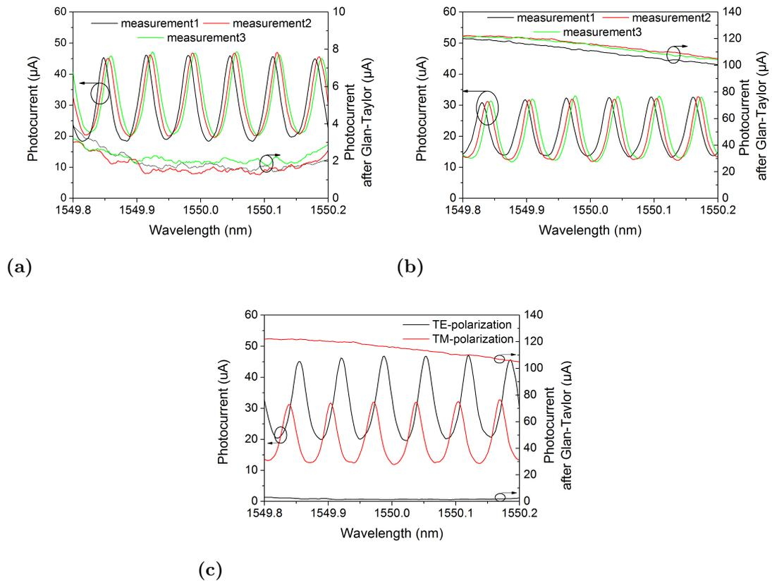
**Figure 6.8:** *Fabry-Pèrot spectrum (1550 nm) of the lower 5400  $\mu\text{m}$  long waveguide and the polarization state of the TLS beam (a) for the TE-polarization, (b) and the TM-polarization, (c) Comparison of both polarizations.*
