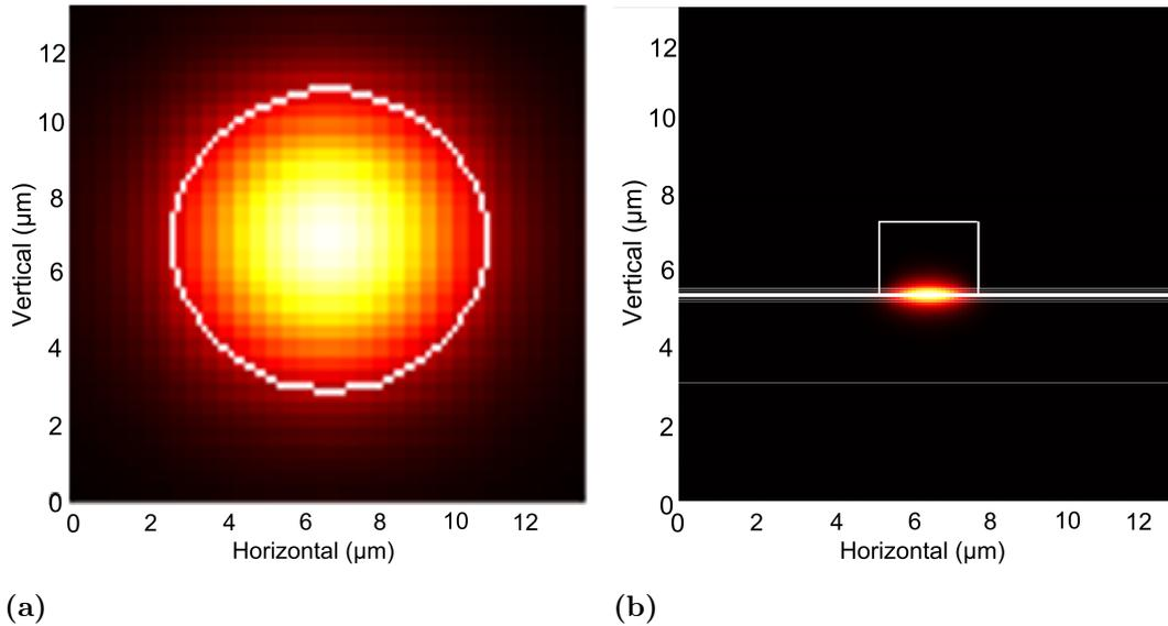
**Figure 1.4:** Intensity of the TE-polarization. (a) 10.4  $\mu\text{m}$  diameter circular spot size of a single mode fiber. (b) 2.4 (horizontal) and 1.0  $\mu\text{m}$  (vertical) spot size of a 1.55  $\mu\text{m}$  laser
