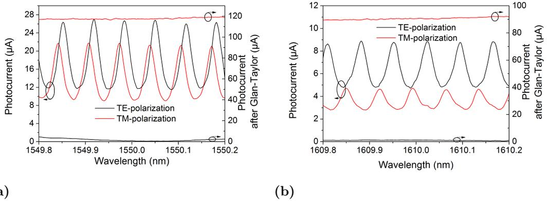
**Figure 6.13:** Fabry-Pérot spectrum of Filter2 (cavity length:  $5400 \mu\text{m}$ ) for both polarizations and the polarization state of the TLS beam (a) at a wavelength of  $1550 \text{ nm}$ , (b) and a wavelength of  $1610 \text{ nm}$ .
