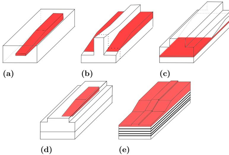
**Figure 3.4:** Vertical taper designs: (a) Vertical down-tapered buried waveguide. (b) Vertical down-tapered ridge waveguide. (c) Vertical overlapping ridge waveguide. (d) Vertical overlapping taper transition from a buried waveguide to a fiber-matched waveguide. (e) Vertical overlapping waveguide taper transition from a ridge waveguide to a fiber-matched waveguide [8].
