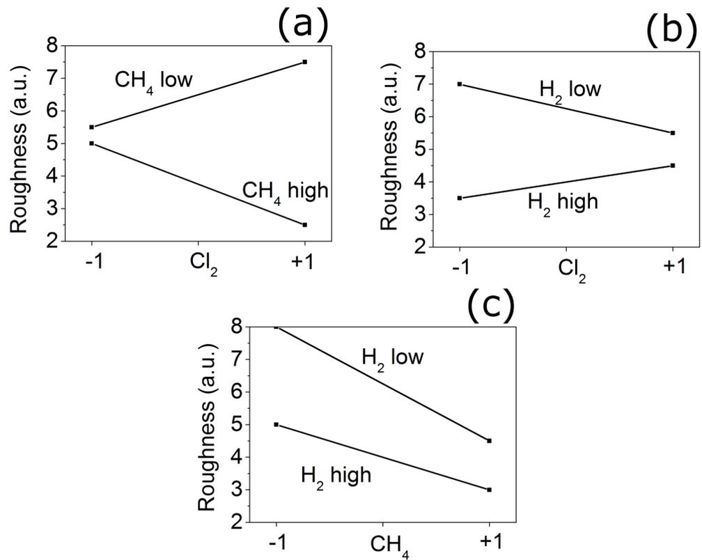
**Figure 9.29:** Interaction plot for the sidewall roughness of  $\text{InP}/\text{InGaAsP}$ , (a) interaction between  $\text{Cl}_2$  and  $\text{CH}_4$ , (b) interaction between  $\text{Cl}_2$  and  $\text{H}_2$ , (c) interaction between  $\text{H}_2$  and  $\text{CH}_4$ .
