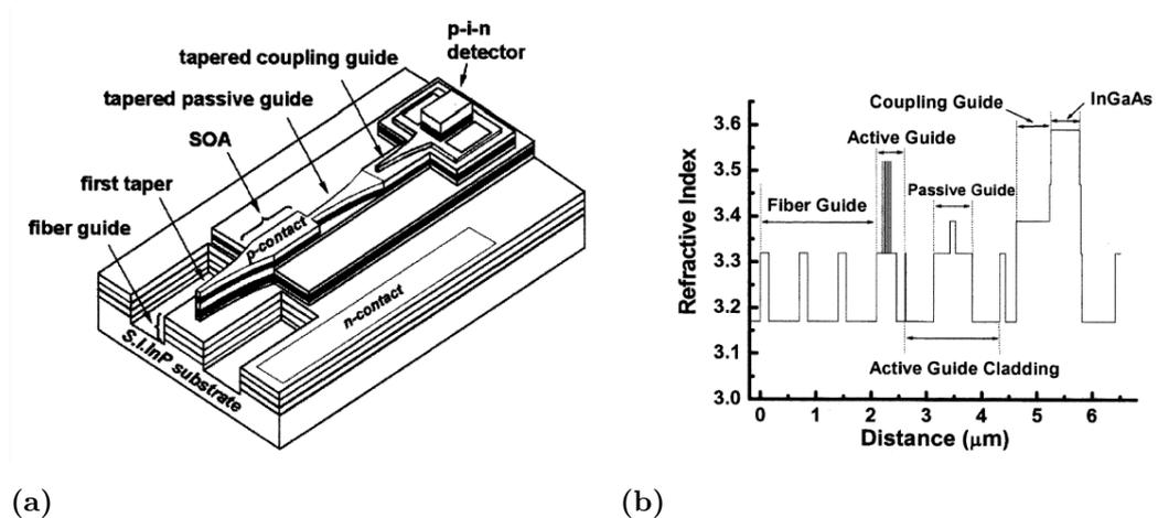
**Figure 3.8:** (a) Three-dimensional schematic view of the integrated ATG SOA/p-i-n chip. (b) Index profile of the SOA/p-i-n epitaxial structure. . The tapered section of the passive guide joins these two parts together [11].
