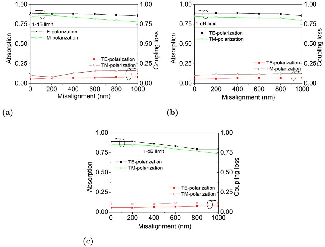
**Figure 7.8:** Absorption efficiency relative to a misalignment (a) of the input to the transition waveguide, (b) of the transition to the coupling waveguide, (c) of the coupling waveguide to the photodiode.
