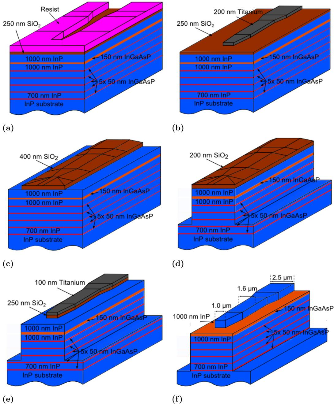
**Figure 9.13:** Consecutive process steps scheme of the chip, (a) after the first lithography step, (b) after the Ti lift-off, (c) after the SiO<sub>2</sub> layers are patterned, (d) after the first III-V material ICP etch, (e) after the overlying SiO<sub>2</sub> mask is removed by an ICP etch, (f) the final ATG structure with SiO<sub>2</sub>/Ti mask removed.
