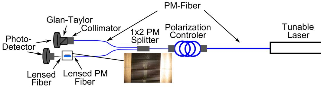
**Figure 6.6:** Schematic of the measurement setup.
