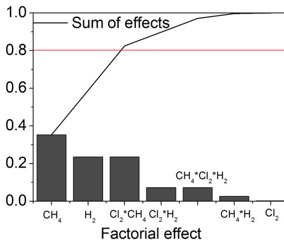
**Figure 9.30:** Sum of squares percentage and the 80 % limit for the sidewall roughness of  $\text{InP}/\text{InGaAsP}$ .
