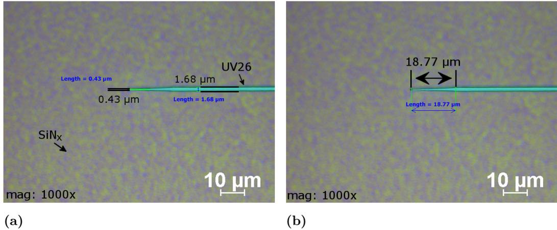
**Figure 9.7:** Microscope images of a properly processed *InP* test chip. The exposure time of UV26 was 11.5 s. (a) ridge width measurement, (b) taper section length measurement.
