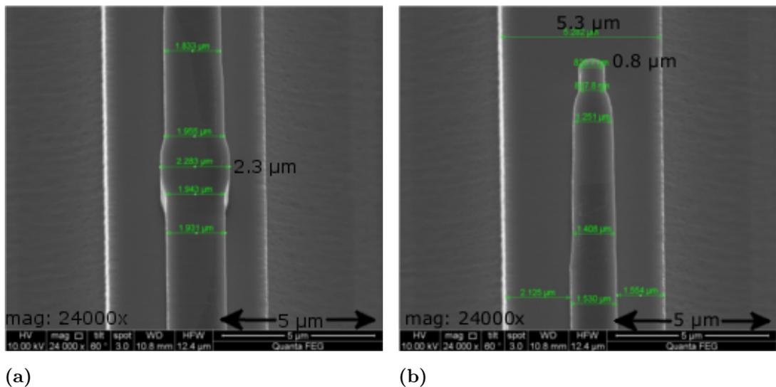
**Figure 9.40:** SEM cross-section images after the process run. (a) Middle section of a 300 nm narrower TM-pass polarizer, (b) Taper end of a TM-pass polarizer with an designed width of  $0.7 \mu\text{m}$ .
