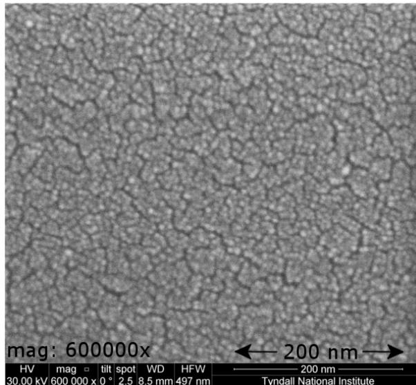
**Figure 9.8:** PECVD deposited  $\text{SiN}_x$  on an *InP* chip.
