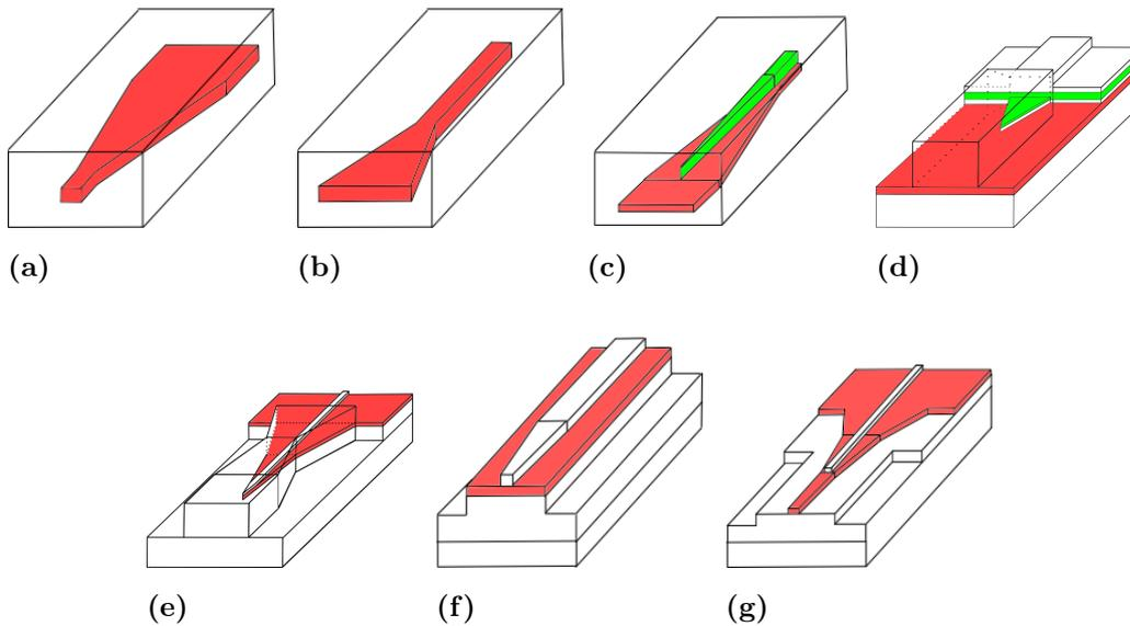
**Figure 3.3:** *Lateral taper designs: (a) Laterally down-tapered buried waveguide (b) Laterally up-tapered waveguide (c) Dual lateral overlapping buried waveguide taper (d) Dual lateral overlapping ridge waveguide taper (e) Nested waveguide taper transition (f) Single lateral taper transition (g) Multisection taper transition [8].*
