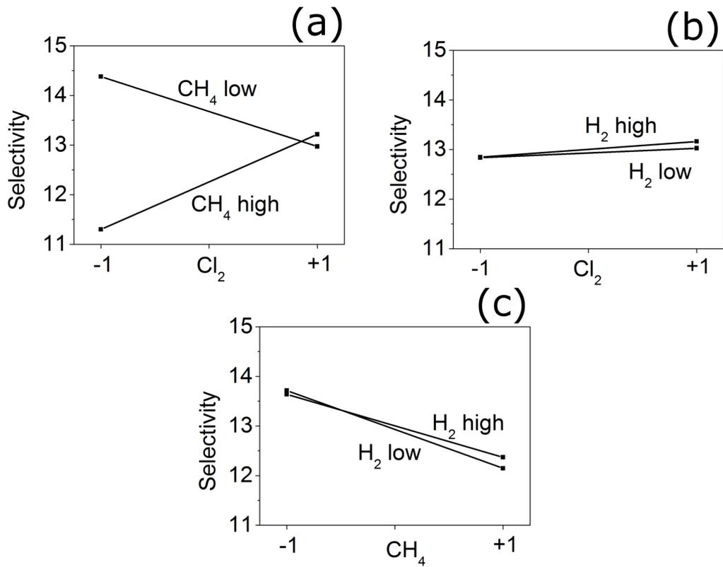
**Figure 9.26:** Interaction plot for the selectivity,  $\text{InP}/\text{InGaAsP}$  to  $\text{SiO}_2$ , (a) interaction between  $\text{Cl}_2$  and  $\text{CH}_4$ , (b) interaction between  $\text{Cl}_2$  and  $\text{H}_2$ , (c) interaction between  $\text{H}_2$  and  $\text{CH}_4$ .
