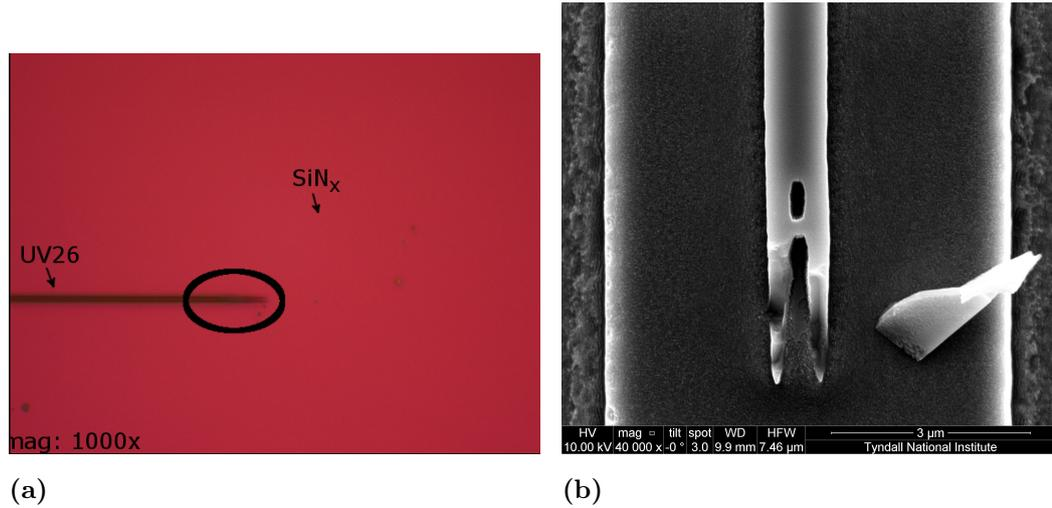
**Figure 9.4:** *InP/InGaAsP chip, (a) microscope image after the first UV26 processing step (b) SEM image of a taper end of a poorly processed chip*
