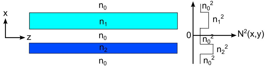
**Figure 2.4:** Directionally coupled optical waveguides.
