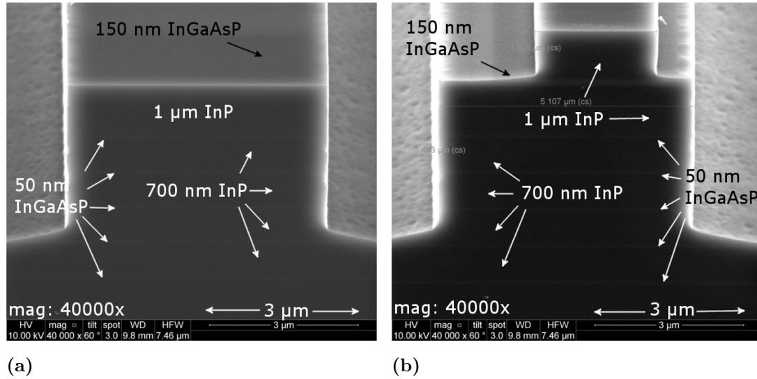
**Figure 6.1:** SEM cross-section images (a) of the single mode input waveguide, (b) of the ATG with an upper InP cladding width of  $2.5 \mu\text{m}$ .
