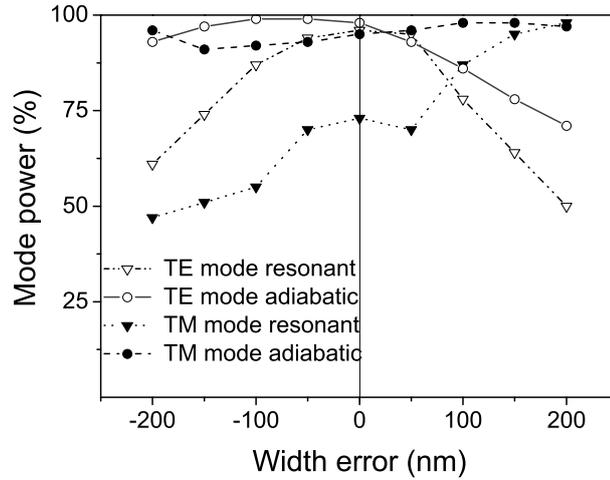
**Figure 4.15:** Mode power in the output mode regarding to a upper waveguide width variation
