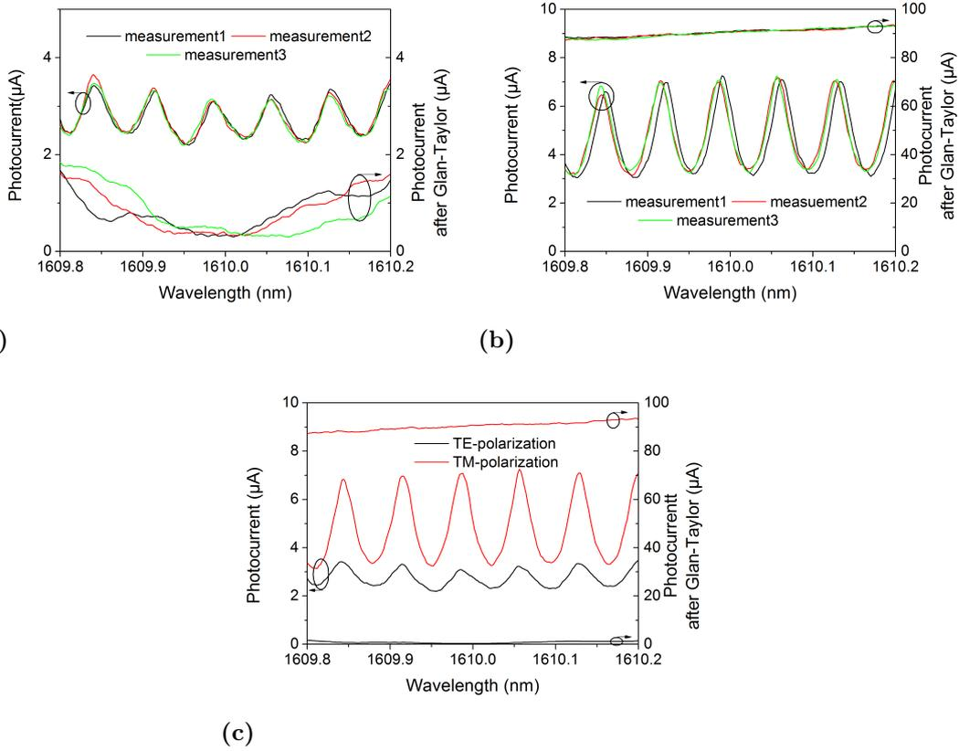
**Figure 6.11:** Fabry-Pérot spectrum (1550 nm) of Filter1 (cavity length: 5400 μm) and the polarization state of the TLS beam (a) for the TE-polarization, (b) and the TM-polarization, (c) comparison of both polarizations.
