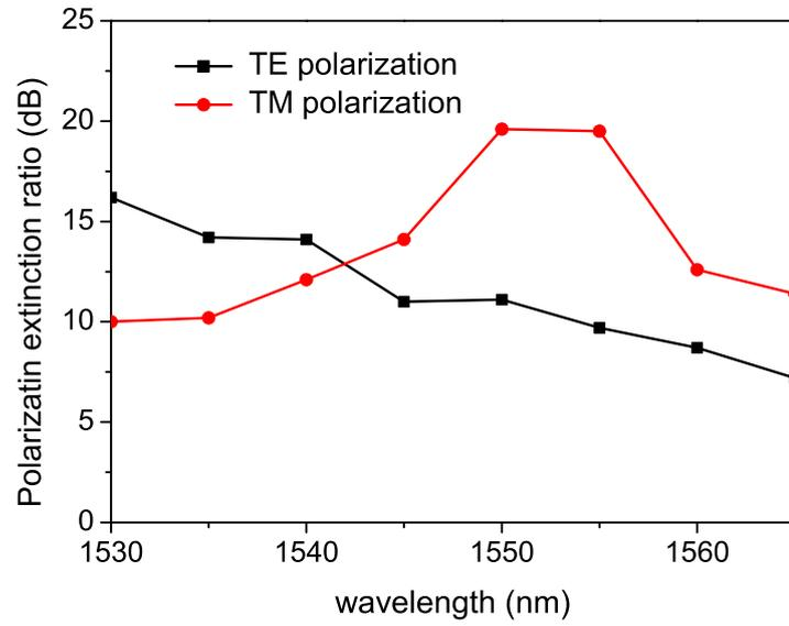
**Figure 5.14:** *Relative power extinction ratio versus wavelength for the polarization splitter*
