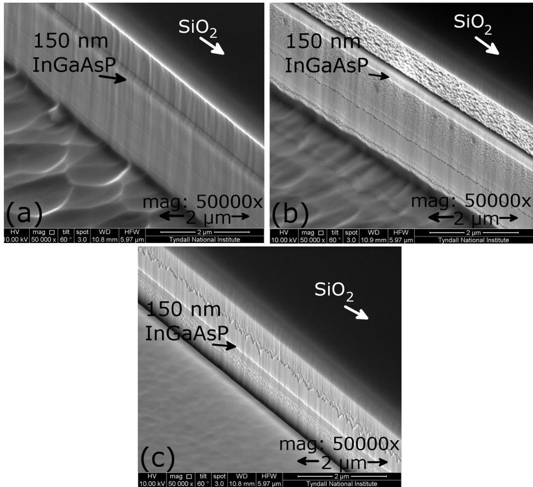
**Figure 9.32:** Cross-section sidewall SEM images, (a) 120 s  $\text{Cl}_2/\text{H}_2 = 10/12$  sccm, (b) 120 s  $\text{Cl}_2/\text{H}_2/\text{Ar} = 10/12/18$  sccm, (c) 120 s  $\text{Cl}_2/\text{CH}_4/\text{H}_2 = 10/18/12$  sccm. The 'scratch' like line is most probably caused by an inferior  $\text{SiO}_2$  mask.
