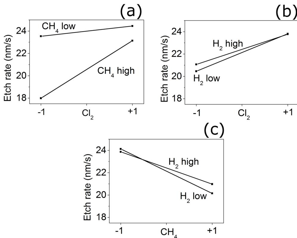
**Figure 9.23:** Interaction plot for the etch rate of *InP/InGaAsP*, (a) interaction between  $\text{Cl}_2$  and  $\text{CH}_4$ , (b) interaction between  $\text{Cl}_2$  and  $\text{H}_2$ , (c) interaction between  $\text{H}_2$  and  $\text{CH}_4$ .
