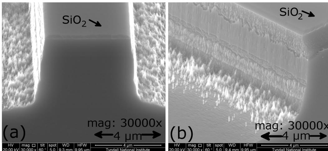
**Figure 9.20:** Cross-section SEM images of the front facet and sidewall of the 195 s etch of  $\text{Cl}_2/\text{CH}_4/\text{H}_2 = 10/7/10$  sccm.
