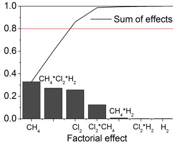
**Figure 9.24:** Sum of squares percentages and the 80 % limit for the etch rate of *InP/InGaAsP*.
