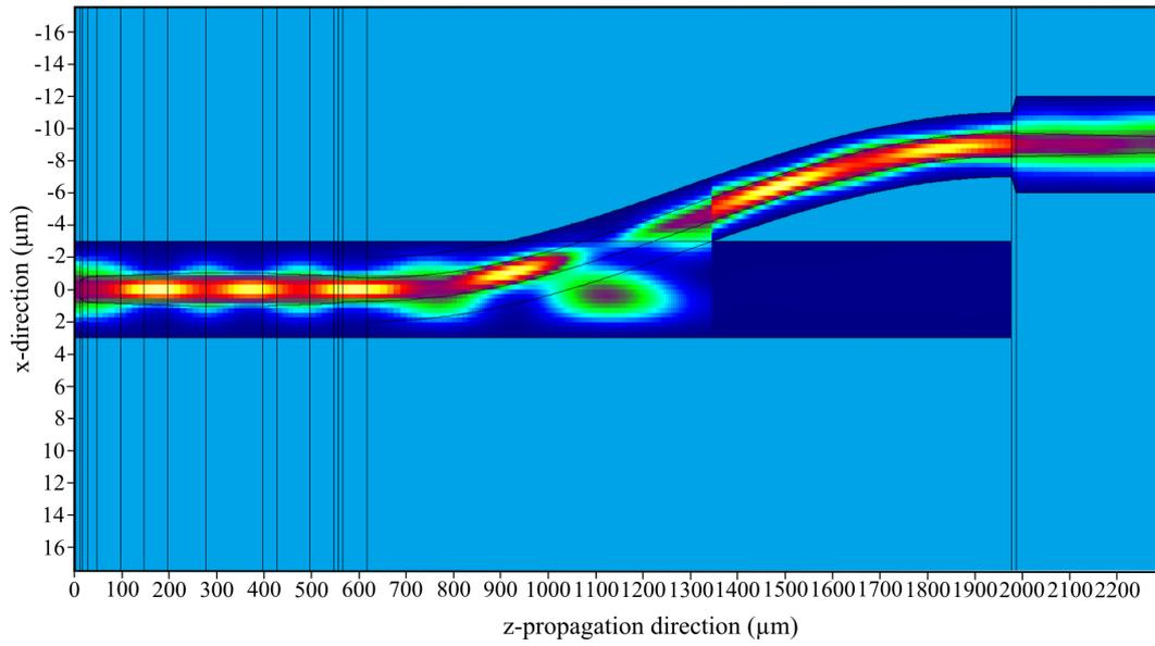
**Figure 5.12:** *Plan view of the intensity distribution for the TE-polarization*
