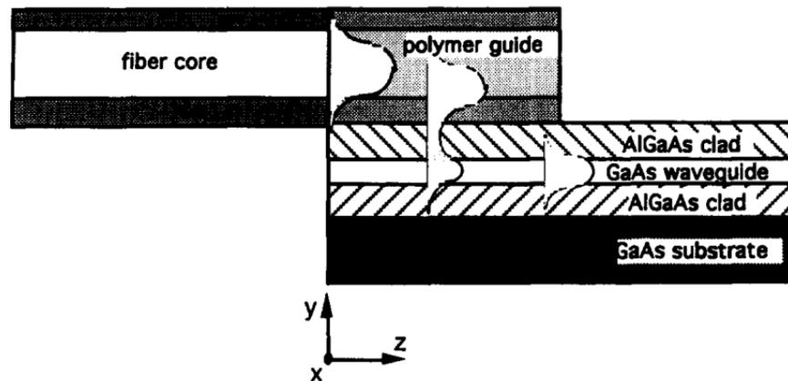
**Figure 3.12:** Basic structure under consideration illustrating the transfer of power from the fiber to the polymer and then to the GaAs waveguide [14].
