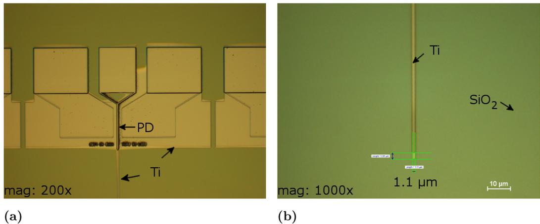
**Figure 9.43:** Microscope images of an InP-test chip after the 200 nm thick Ti-lift-off. (a) PDs with SSC, (b) SSC upper waveguide end
