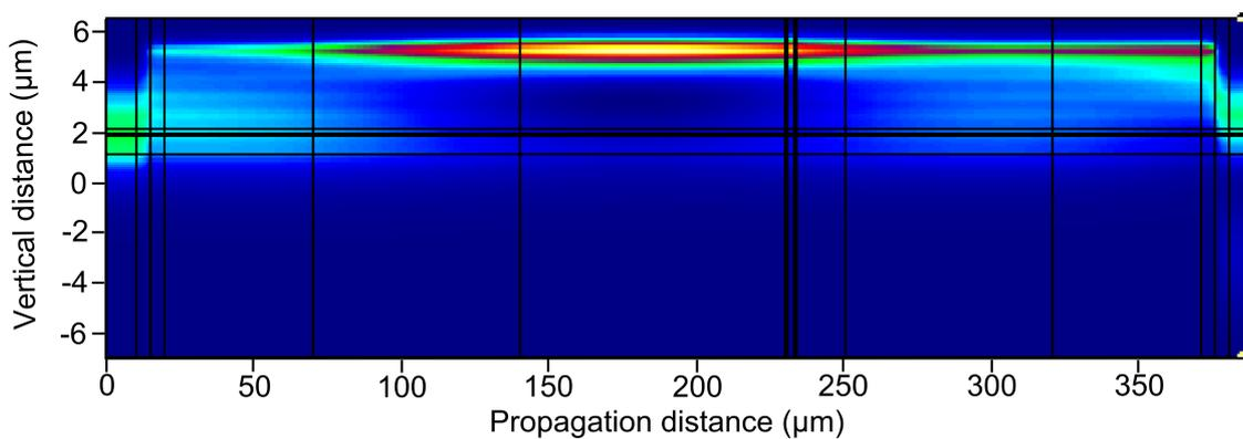
**Figure 6.3:** Side view of the intensity distribution of the TM-field, the input is on the left side in the lower waveguide. The vertical lines correspond to section boundaries. In both cases the taper start width is 700 nm. The total taper width is reduced by 300 nm compared to the ideal case in Chapter 5.
