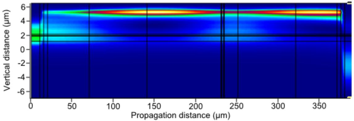
**Figure 6.5:** Side view of the intensity distribution of the TM-field, the input is on the left side in the lower waveguide. The vertical lines correspond to section boundaries. In both cases the taper start width is 900 nm. The total taper width is reduced by 100 nm compared to the ideal case in Chapter 5.
