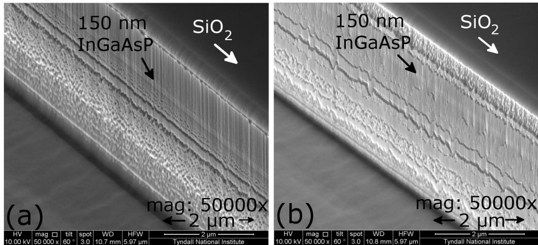
**Figure 9.35:** Cross-section SEM images of the sidewalls, etch ( $\text{Cl}_2/\text{CH}_4/\text{H}_2 = 10/18/12$  sccm,  $\text{InP}/\text{InGaAsP}$ ), (a) run 2, 180 s, (b) run 1, 210 s. The 'scratch' like lines in (a) and (b) are most probably caused by an inferior  $\text{SiO}_2$  mask.
