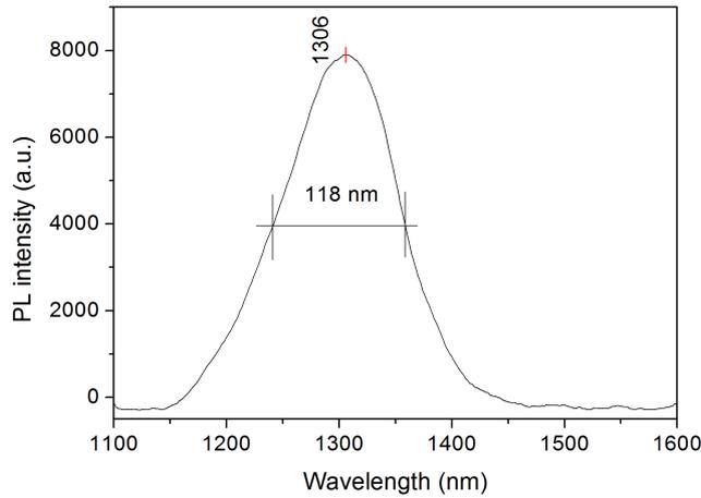
**Figure 8.8:** Photoluminescent measurement of chip A1034.
