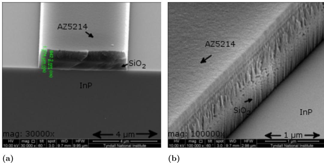
**Figure 9.18:** Cross-section SEM images of AZ5214 after an SiO<sub>2</sub> etch. (a) front facet, (b) sidewall.
