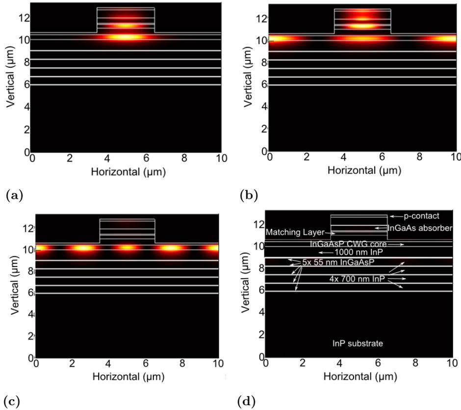
**Figure 7.3:** Excited mode intensity distribution at the intersection SSC-PD (a) lowest order mode with an overlap between the CWG and absorber, (b) next higher order mode with an overlap between the CWG and absorber, (c) higher order mode with hardly any overlap between the CWG and absorber, (d) Cross section view of the layers of the SSC and PD.
