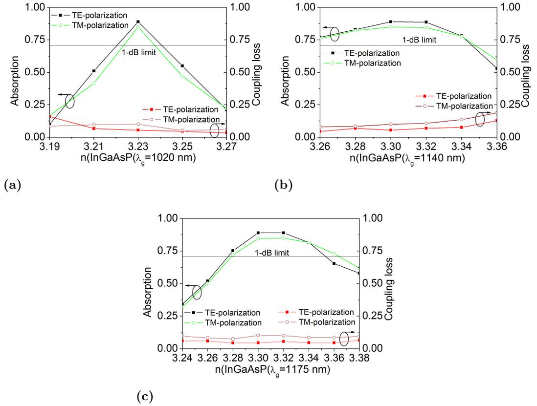
**Figure 7.10:** Absorption efficiency relative to a refractive index variation of (a) InGaAsP ( $\lambda_g = 1020 \text{ nm}$ ), (b) InGaAsP ( $\lambda_g = 1140 \text{ nm}$ ), (c) InGaAsP ( $\lambda_g = 1175 \text{ nm}$ ).
