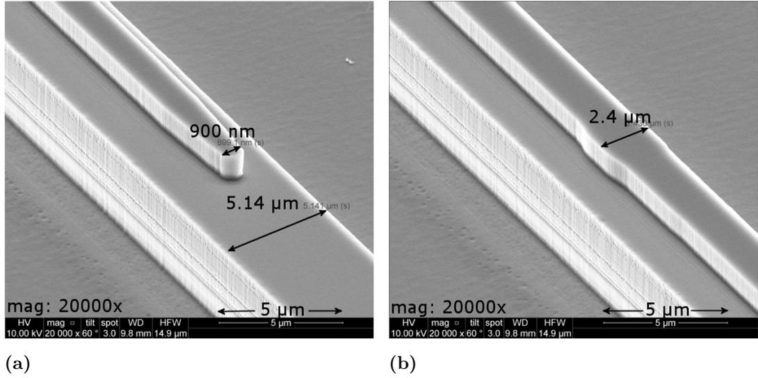
**Figure 6.12:** Cross-section SEM images of Filter2 (a) of the taper end of the polarizer, (b) of the center of Filter2.
