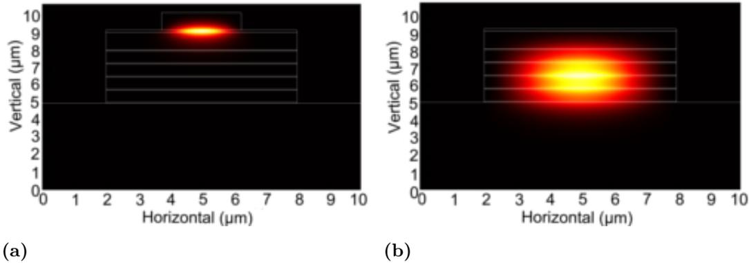
**Figure 4.3:** *TE mode intensity profile, (a) ridge width  $2.5 \mu\text{m}$ , lower waveguide width  $6 \mu\text{m}$ : optical field width ( $1/e^2$ ) horizontal:  $2.2 \mu\text{m}$ , width vertical ( $1/e^2$ ):  $1.2 \mu\text{m}$ , (b): lower waveguide width  $6 \mu\text{m}$ : optical field width ( $1/e^2$ ) horizontal:  $4.6 \mu\text{m}$ , width vertical ( $1/e^2$ ):  $4.3 \mu\text{m}$ ,*
