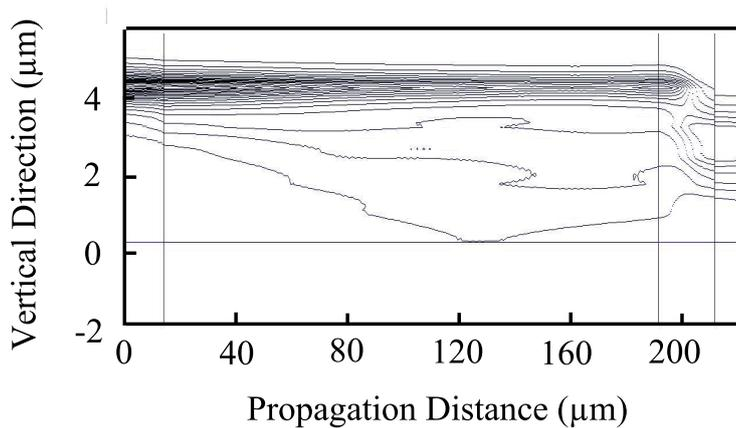
**Figure 4.17:** Side view of the 200 nm wider resonant coupler, contour plot of the field intensity distribution. The vertical lines correspond to section boundaries.
