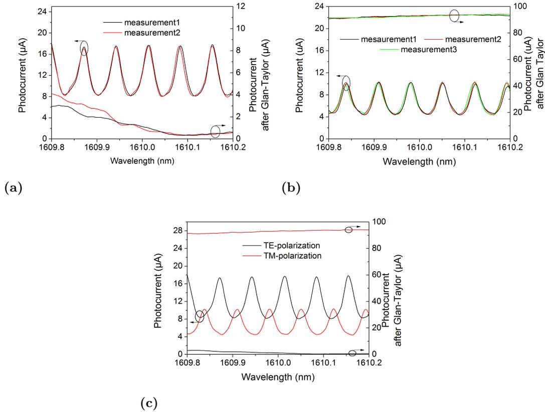
**Figure 6.9:** *Fabry-Pèrot spectrum (1610 nm) of the lower waveguide and the polarization state of the TLS beam (a) for the TE-polarization, (b) and the TM-polarization, (c) Comparison of both polarizations.*
