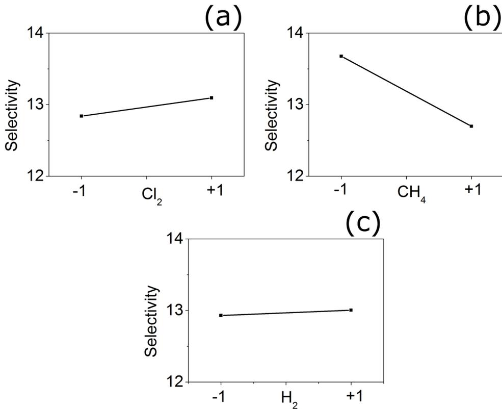
**Figure 9.25:** Main effects plot for the selectivity, InP/InGaAsP to SiO<sub>2</sub>, (a) main effect of Cl<sub>2</sub>, (b) main effect of CH<sub>4</sub>, (c) main effect of H<sub>2</sub>.
