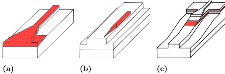
**Figure 3.5:** *Combined vertical and lateral taper designs: (a) Combined lateral and vertical ridge waveguide taper. (b) 2-D overlapping waveguide taper transition from a buried waveguide to a fiber-matched waveguide. (c) Overlapping waveguide taper transition with two sections from a ridge waveguide to a fiber matched waveguide [8].*
