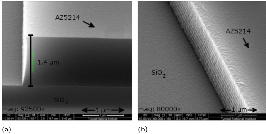
**Figure 9.17:** Cross-section SEM images of AZ5214 exposed and developed for 7.5 s and 25 s respectively. (a) height measurement, (b) sidewall.
