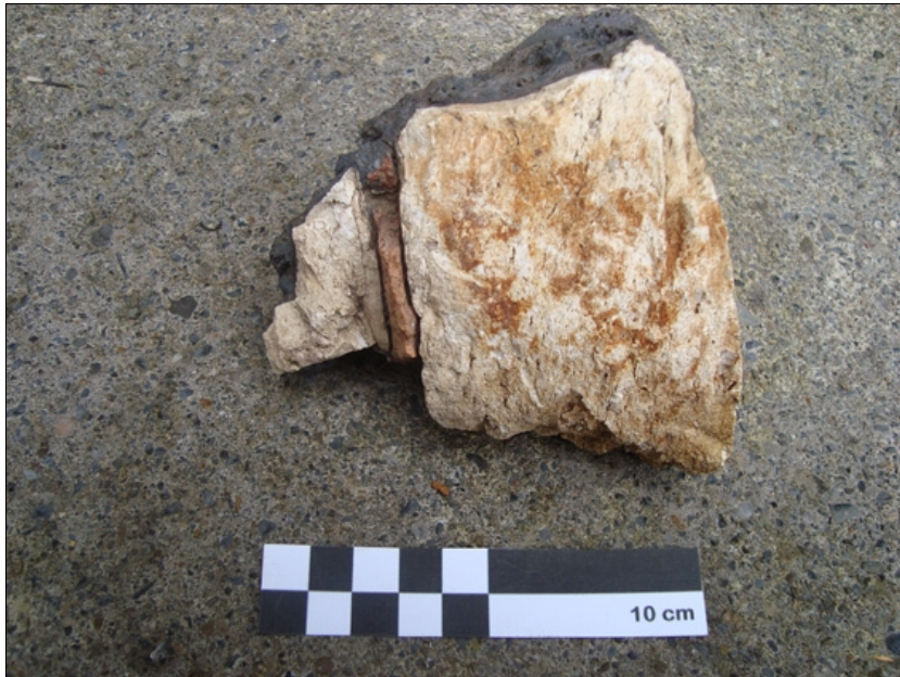
Fig. S.30 Mallow, Quartertown, Co. Cork. Finery slag with adhering stone-work
