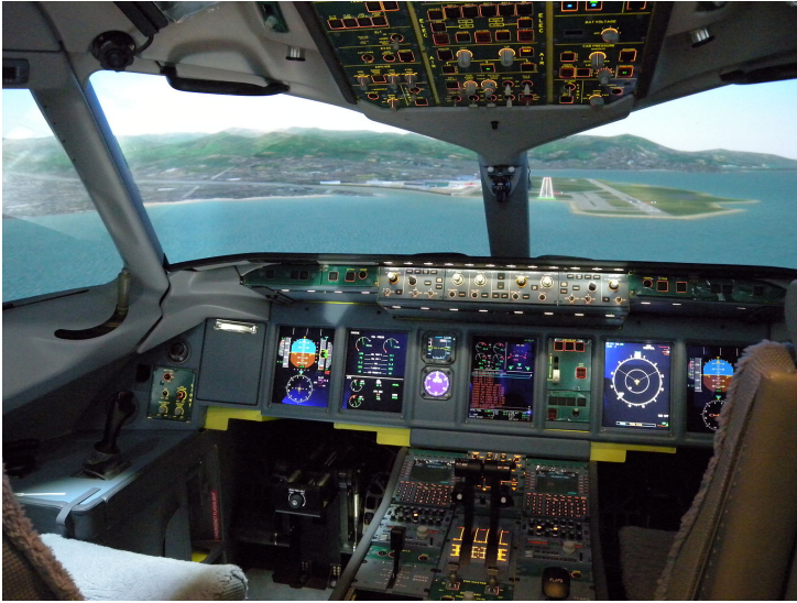
Fig. 7 Flight simulators are experimental simulations that facilitate training and study of the behavior of pilots in pre-programmed scenarios. Image credits: SuperJet International, distributed under CC BY-SA 2.0 Source: SuperJet International (2011)
