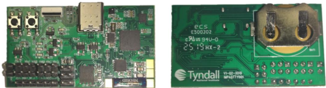
Figure 14 - Evaluation IMPAQT PCB of tag fabricated, front and back respectively.
