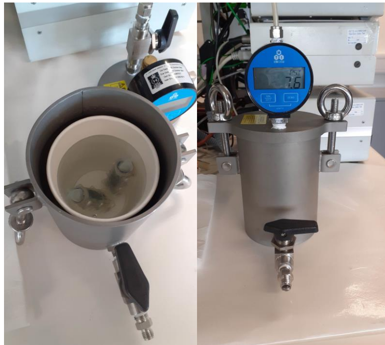
Figure 36 - Test setup for the pressure sensor test in water.
