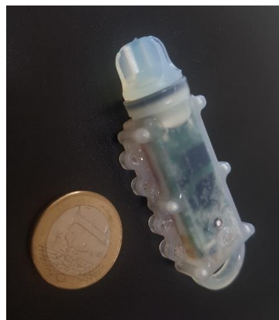
Figure 30 - Final embedded system for seaweed monitoring encapsulated.
