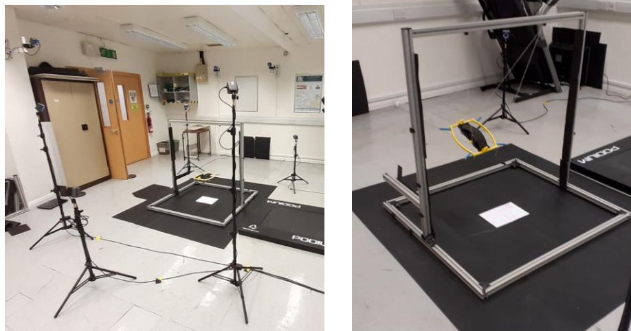
Figure 32 - (a) Pendulum in the area covered by the Optitrack cameras; (b) Pendulum mounted in the aluminium frame. The reflective markers were placed in the four corners of the pendulum base to track the oscillation of the whole system.
