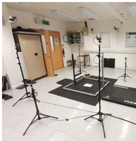
Figure 32 - (a) Pendulum in the area covered by the Optitrack cameras; (b) Pendulum mounted in the aluminium frame. The reflective markers were placed in the four corners of the pendulum base to track the oscillation of the whole system.
