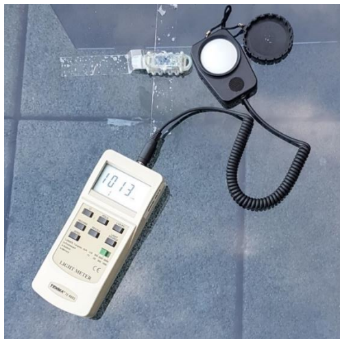
Figure 39 - Light measurement calibration of Aquabit
