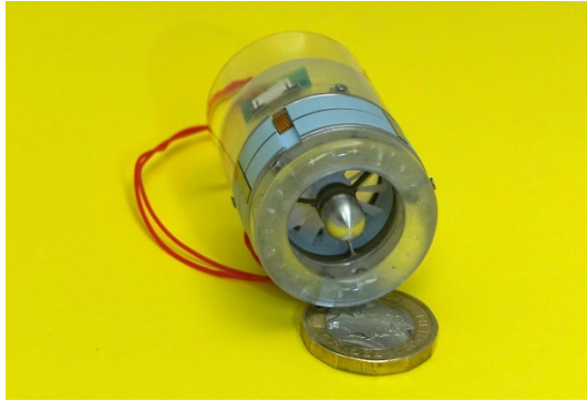
(a) (b) Figure 10— 2 cm Diameter Micro-Wind Turbine (MWT) EH for Duct Monitoring: (a) Prototype Device with British £1 Coin for Scale; (b) Measured Variation of Electrical Output Power with Wind-Speed (Theoretical Curves for 5% and 2% Overall Efficiency)
