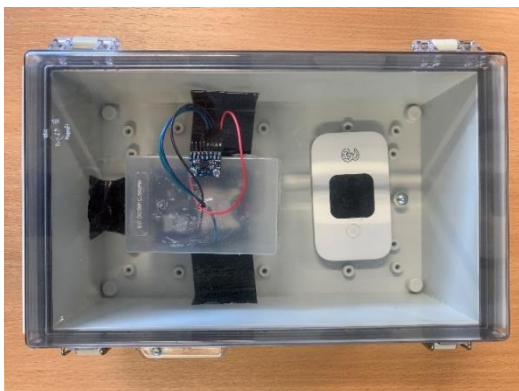
Figure 4. 36 Sensor box applied to the Connolly Street slope
