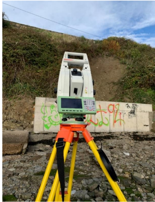
Figure 4. 18 Laser scanner in action at the Connolly Street slope, Cobh
