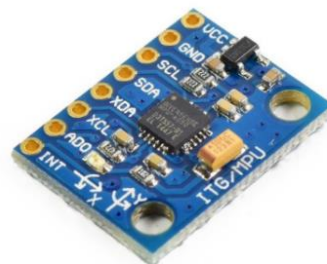
Figure 4. 25 Inertial measurement sensor (20)
