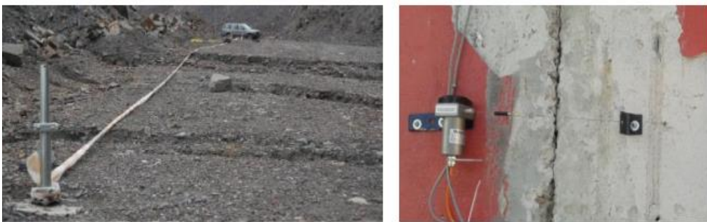
Figure 3. 8 Extensometer in action (10)
