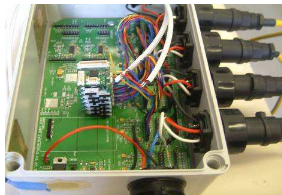
Figure 2: Multi-sensor interface board with sensors
