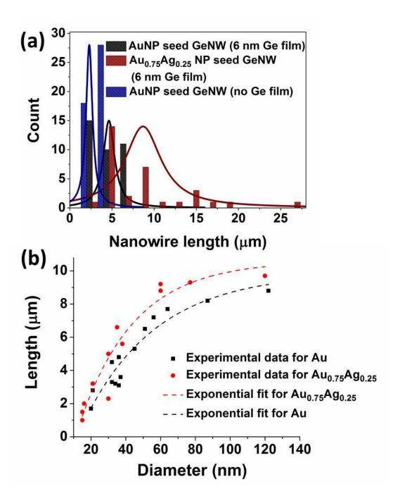
**Figure 5.** Plots of nanowire length vs growth rate showing the applicability of the Gibbs-Thompson effect. (a) Length distribution curves comparing the lengths of Ge nanowires grown from Au and  $Au_{0.75}Ag_{0.25}$  nanoparticles. (b) Plot of nanowire length as a function of diameter for nanowires grown from Au and  $Au_{0.75}Ag_{0.25}$  nanoparticles.
