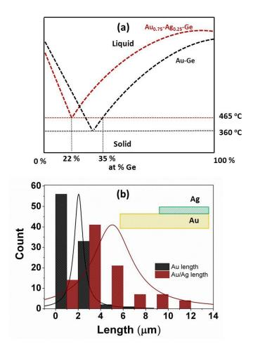
**Figure 3.** Diameter distributions highlighting the difference in lengths of nanowires grown from a Au film and a Au-Ge bilayer. (a) Phase diagram showing the shift in equilibrium concentration in the Au-Ag-Ge ternary alloy system when compared with the Au-Ge binary system. (b) Length distribution data comparing the lengths between nanowires grown from a Au film and a Au-Ag bilayer.
