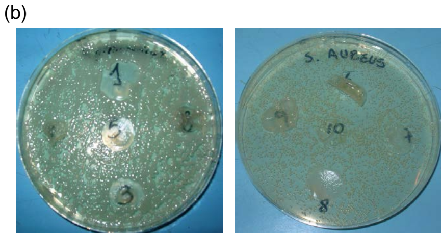
FIGURE 4. (a) Diffusion disc results of chitosan composite films and (b) inhibition halo formation, against Klebsiella pneumoniae (left) and Staphylococcus aureus (right). Films that were case without plasticizing additives are more difficult to manipulate and had a tendency to roll into a tubular shape after being added to the serum and such films exhibited the greatest dimensional change due to swelling.
