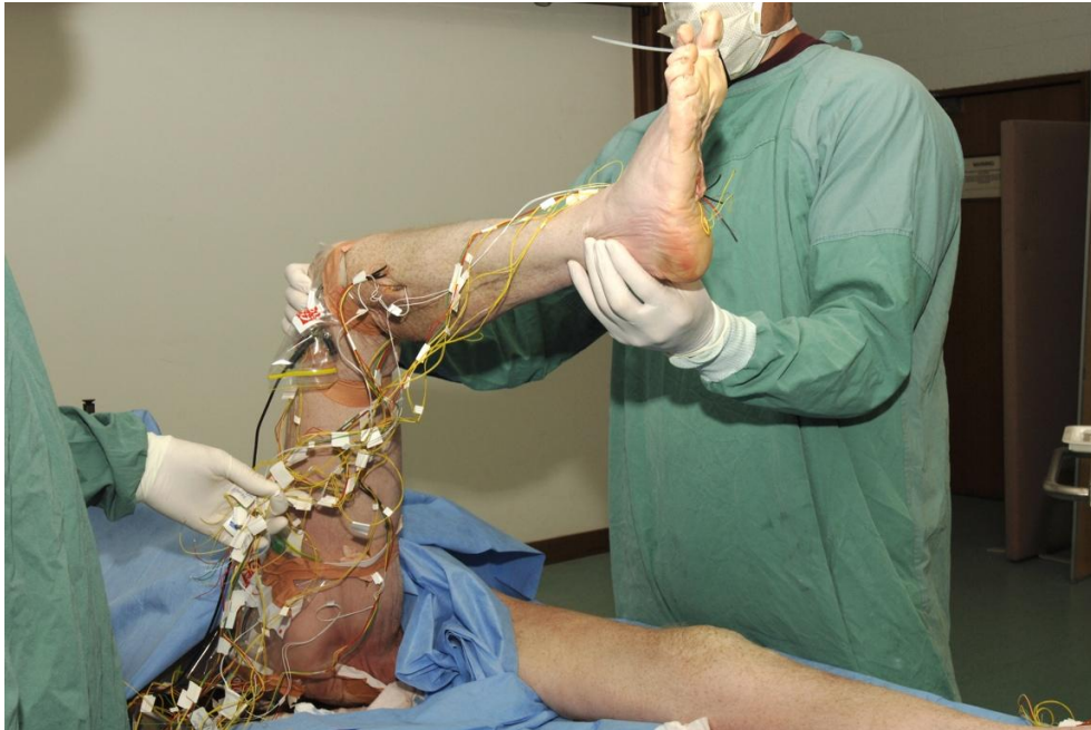
Figure 5.3: Instrumented (multiple microstrain gauges and electronic goniometer) cadaveric limb in completion of HIP test.
