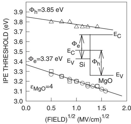
FIG. 4. Schottky plot of the electron ( $\circ, \square$ ) and hole ( $\triangle$ ) IPE thresholds measured in (100)Si/MgO/Au samples with as-deposited ( $\circ, \triangle$ ) and crystallized ( $\square, \triangle$ ) MgO layers. The insert shows a schematic of the Si/MgO interface band diagram with the electron ( $\Phi_e$ ) and hole ( $\Phi_h$ ) IPE barriers indicated by arrows.
