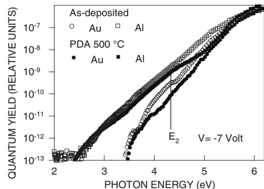
FIG. 3. Logarithmic plot of the IPE quantum yield as a function of photon energy measured in (100)Si/MgO/Au samples with as-deposited (open symbols) and crystallized (filled symbols) MgO under  $-7$  V bias applied to the Au (circles) or Al (squares) electrode. The vertical line marks the onset of the  $E_2$  direct optical transition in the Si substrate crystal.
