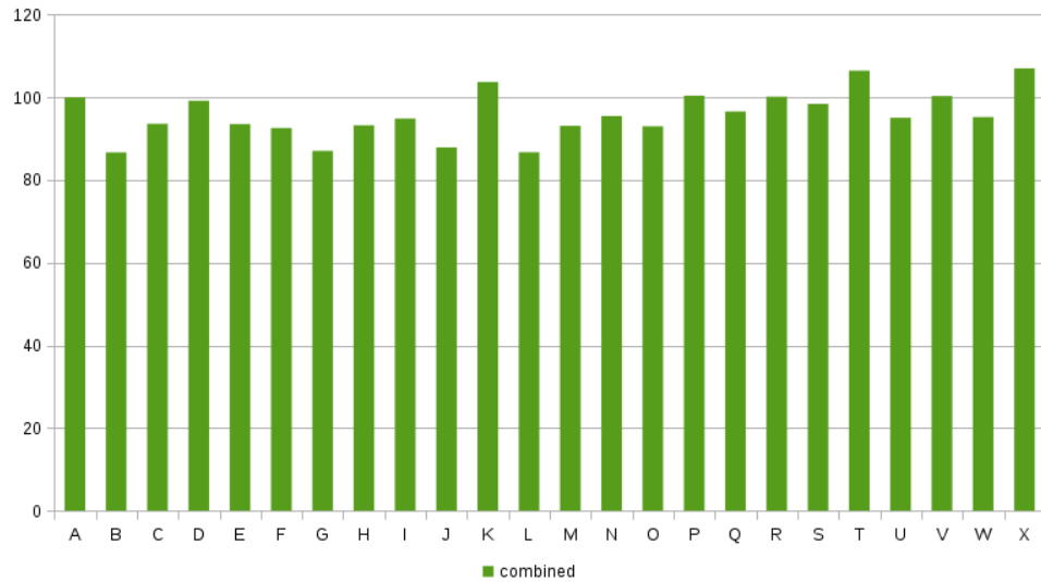
Figure 5.9: Configuration performance for the dbench workload of combined sequential and random accesses with weights applied.
