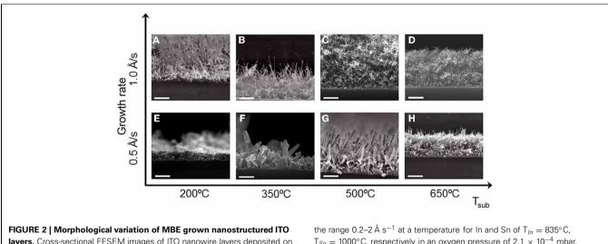
**layers.** Cross-sectional FESEM images of ITO nanowire layers deposited on silicon as a function of deposition rate and temperature of the Sn precursor. A transition from film growth to NWs arrays with decreasing average NW diameter is clearly observed with increasing temperature and deposition rate. For all structures, the In:Sn ratio (90:10) was evaporated at growth rates in
