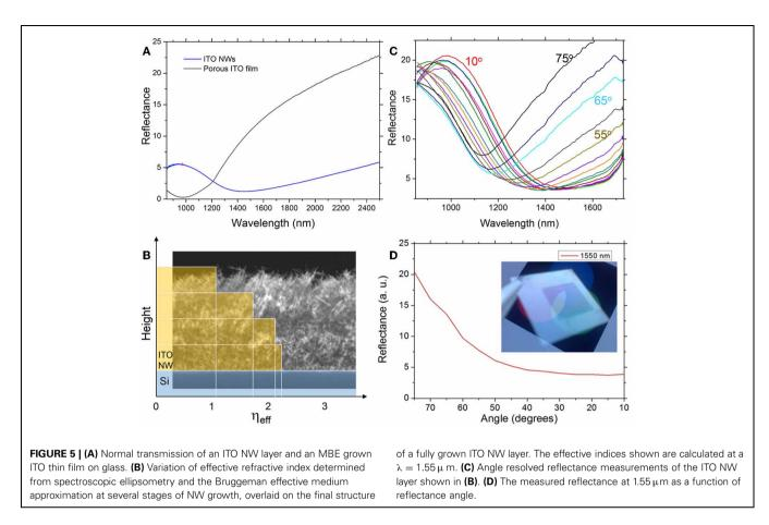
on the NW size, distribution, branching and overall optical morphology. The low refractive index NW layer is optically specular and exhibits a darker surface, confirming the absence of Fresnel reflection over a broad spectral width. This is particularly important for LED applications because of the isotropic emission from the active region and the fact that reflection phenomena can limit the light-extraction efficiency (27, 38, 39).
