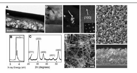
**FIGURE 4 | (A)** TEM image of a region of the ITO NW layer at early stages of NW growth showing the porous nature of the deposit stemming from the seed layer on the Si surface. **(B)** Large area EDX spectrum acquired after early stages of NW growth showing the In and Sn Ledge lines, O and Si substrate lines of (In<sub>1.875</sub>Sn<sub>0.125</sub>)O<sub>3</sub>. **(C)** XRD pattern for early stages of NW growth indexed to the (In<sub>1.875</sub>Sn<sub>0.125</sub>)O<sub>3</sub>
