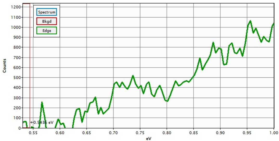
Figure S16: Enlarged view of the sub 1.0 eV region of the EELS Spectra. The bandedge can be clearly seen at approx. 0.61 – 0.62 eV.
