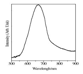
Fig. 5 PL spectrum of Si nanopillar arrays on Si substrate.
