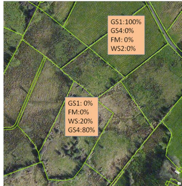
Figure 3.2. Example of land cover percentages apportioned to enclosed Prime2 objects (where GS1 is dry calcareous and neutral grassland, GS4 is wet grassland, GM is marsh and WS2 is immature woodland).
