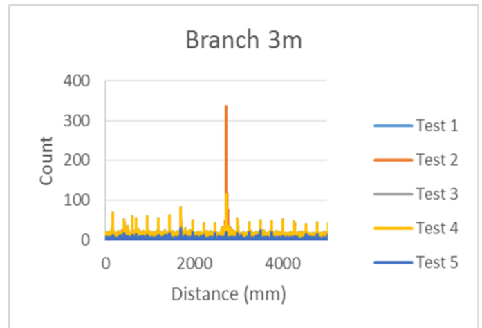
Fig. 7 Histogram Output for a branch 3m from sensor
