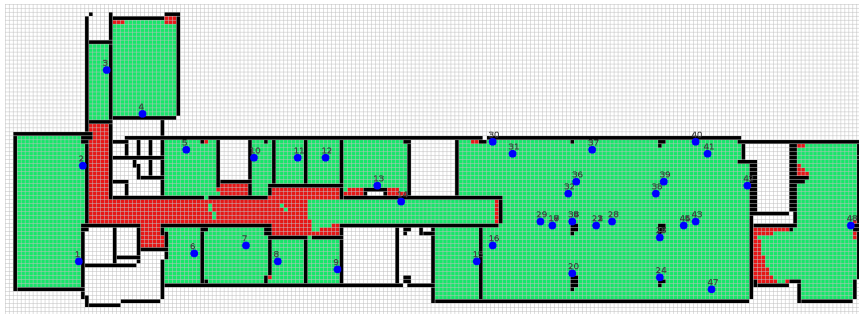
Figure 5. WSN deployment on the first floor of the Cork Institute of Technology (CIT-1).
