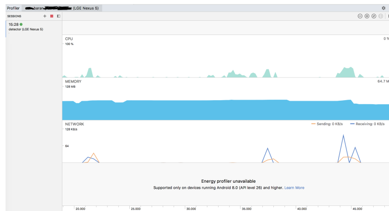
Figure D.4: The hardware usage of the device when Baran data collection service is running
