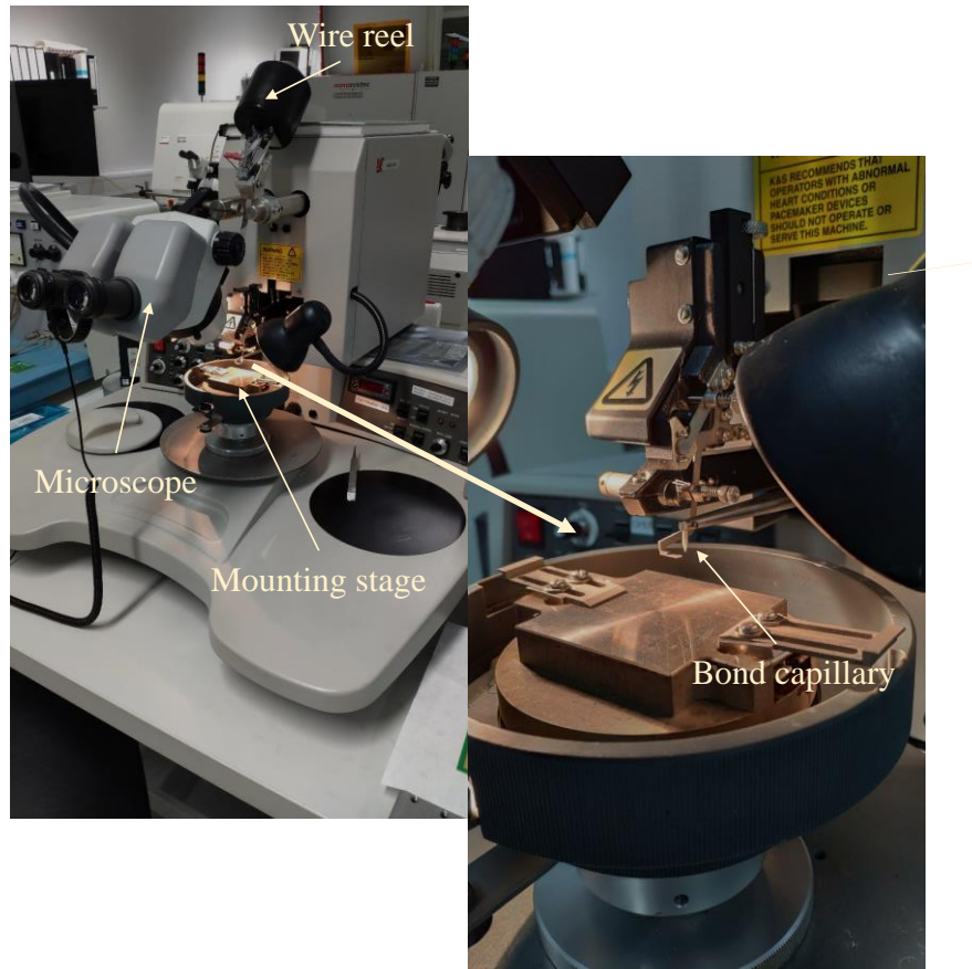
Fig. A2. Manual wire bonder by K&S used for Au stud bumping on device bond pads and wire bonding to connect device to interposer or test board. Typical wire diameter used on the system is 0.8 and 1.0 mil.
