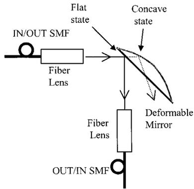
Fig. 4 VOA design using two single fiber lenses.
