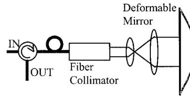
Fig. 6 High resolution VOA design using the focusing effect of the deformable mirror.
