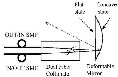
**Fig. 2** Compact VOA design with dual fiber collimator and micromachined deformable mirror using the tilt effect.
