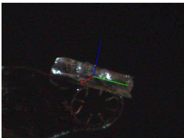
Figure 2: Lattice orientation of 5.MeOH showing preferential growth along the crystallographic b axis.
