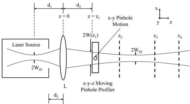
FIG. 1. The traditional moving optics beam analyzer method to determine the  $M^2$  beam parameter. In the shown analyzer operation, the profiler imaging plane is moved along the  $z$  axis and the beam waists are measured at multiple planes like  $z_1, z_2, z_3, z_4$ , etc. The lens  $L$  has a fixed position and focal length  $F$ .
