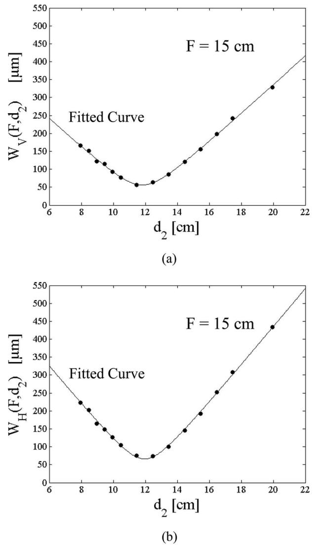
FIG. 3. Characterization of the multimode laser beam using the classic prior-art method with physical motion of the analyzer (i.e., the DMD) to measure the second-moment irradiance beam radii  $W_V(F, d_2)$  and  $W_H(F, d_2)$  at different  $d_2$  positions. Data plots are for (a) the vertical (or  $y$  direction) beam waist and (b) the horizontal (or  $x$  direction) beam waist.
