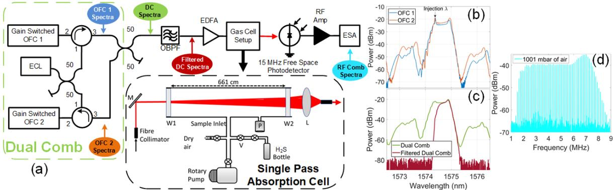
Figure 1: (a) DCS setup used to detect H<sub>2</sub>S in the near-infrared. Optical spectra taken at the points indicated in the experimental setup; (b) OFC1 (blue line) and OFC2 (orange line) and (c) DC output before (green line) and after the optical bandpass filter (OBPF) (red line). (d) Background RF beat tone spectrum taken with the ESA. W1, W2: optical windows; L: Achromatic lens; P: Absolute pressure sensor; V: valve; M: mirror.
