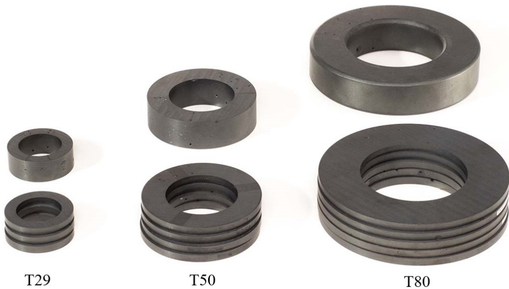
Figure 130. Cores used to test the core size effect on lamination performance.
