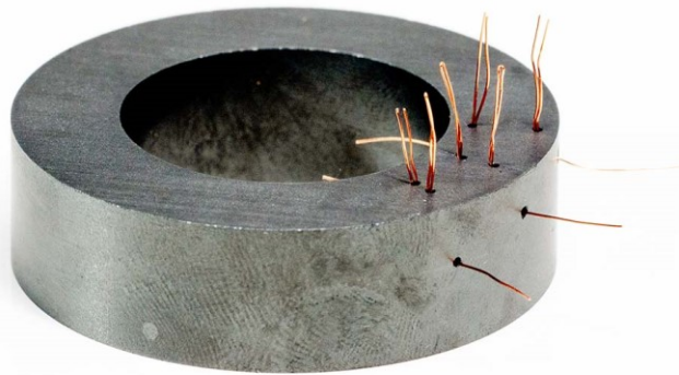
Figure 108. Tested core with sense winding.
