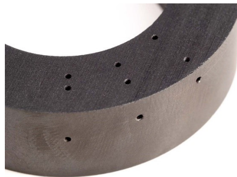
Figure 107. Tested core with drilled three sets of holes.
