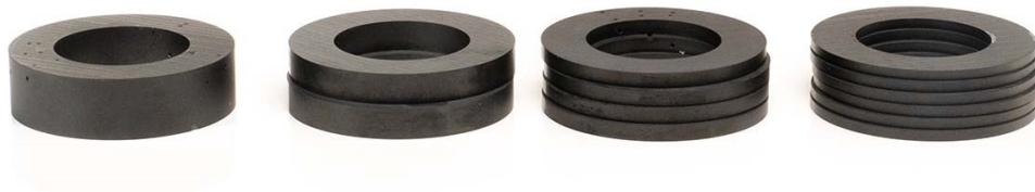
Figure 118. T50 cores to test lamination thickness impact on core performance.
