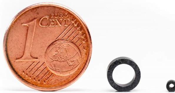
Figure 22. T6 and T2 cores to test complex permeability characteristic.
