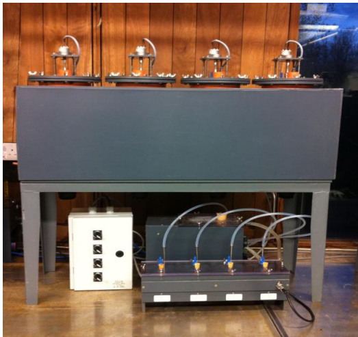
Figure A1 Semi-continuous AD digestion system consisting of 5 L reactors and tipping bucket measuring device
