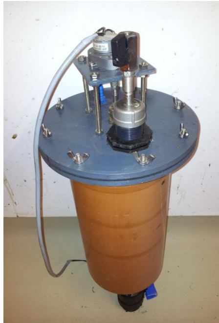
Figure 8.2 Continuously stirred tank reactor (5L) used for semi continuous trial
