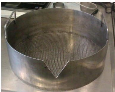
Figure 7.5: V notch weir cut into biomass holding cage
