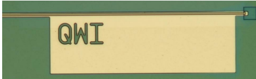
Figure 3.15 Microscopic picture after p metal lift-off process step.
