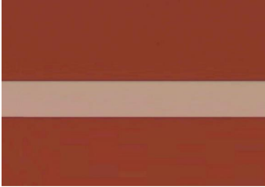
Figure 3.8 Using standard photolithography to define the QWI zone (Tan color is QWI zone, dark red color is non-QWI zone).
