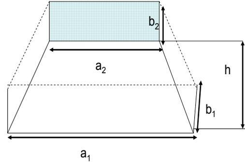
Fig.4. Schematic of trapezoid where  $a_1$ ,  $a_2$  are the lengths,  $b_1$  and  $b_2$  widths and  $h$  the height. In the trapezoid,  $a_2 \times b_2$  represents the chip pad while  $a_1 \times b_1$  represents board pad and  $h$  is stand-off height
