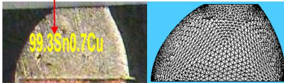
**Fig. 2.** Cross-section of ratio  $\text{chip}_{\text{pad}}/\text{sub}_{\text{pad}}$  0.6 and its corresponding Surface Evolver predicted shape.
