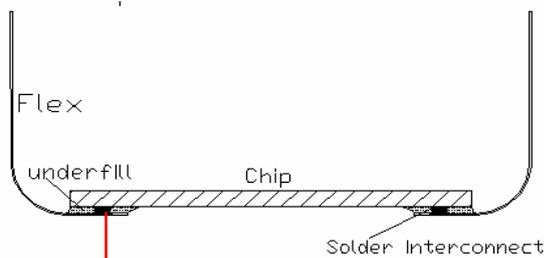
**Fig. 1.** Schematic of FCOH
