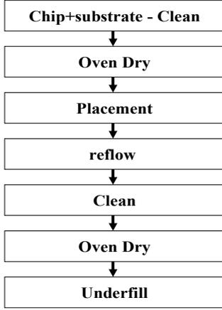
Fig. 3. Process flow for flip chip assembly
