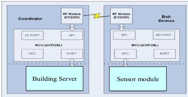
Figure 1. Zigbee Module H/W Architecture
