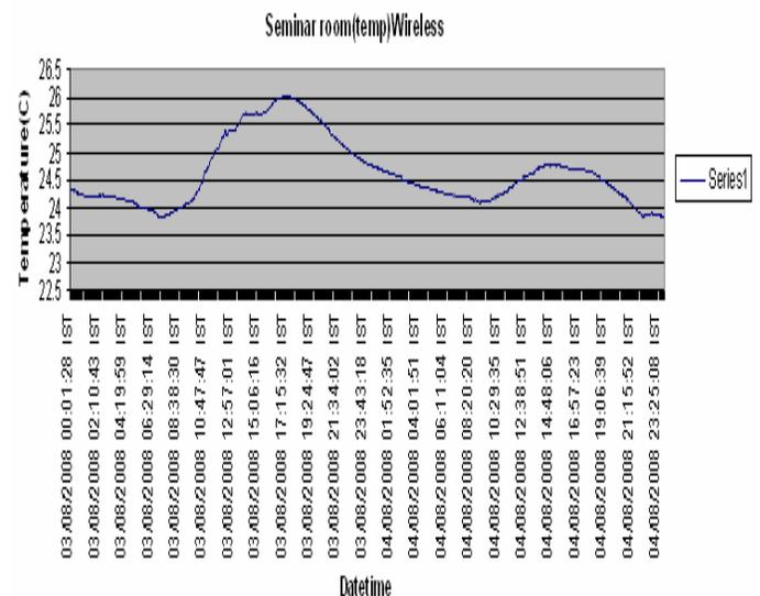
Figure 12. Seminar Room Temperature Statistics for Wireless Sensors
