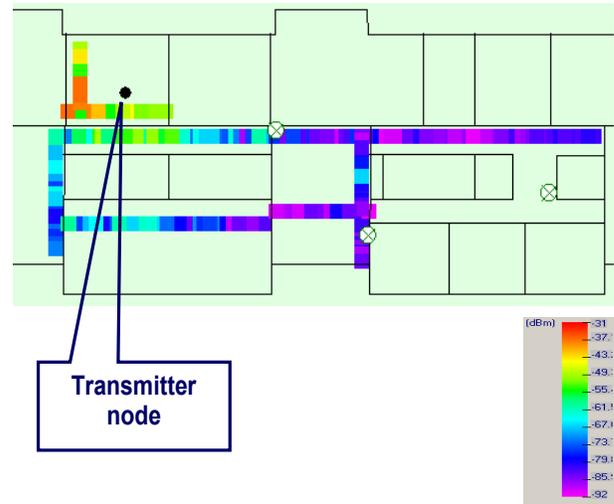
Figure 3. Measured RSSI level for the First Floor
