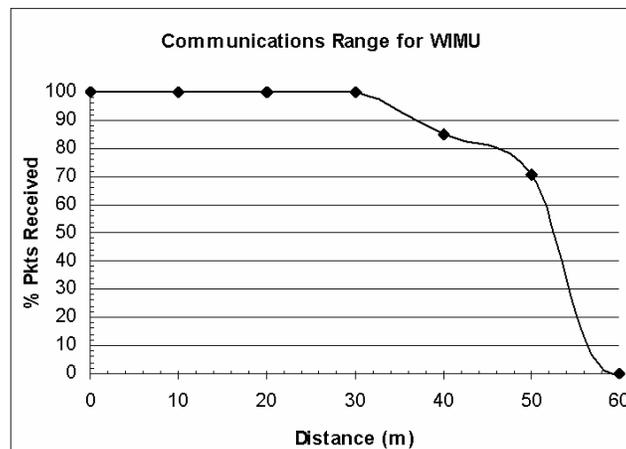
Figure.20: Packet Loss Measurements
