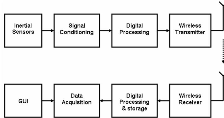
Figure. 2: Wireless Inertial Sensing System Block Diagram.
