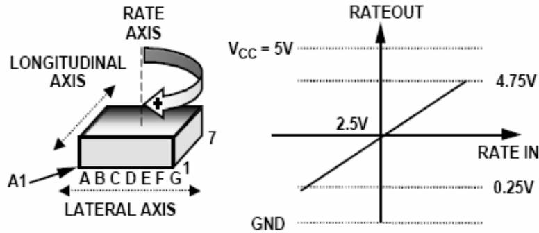
Figure. 6: RATEOUT Signal Increases with Clockwise Rotation [16].
