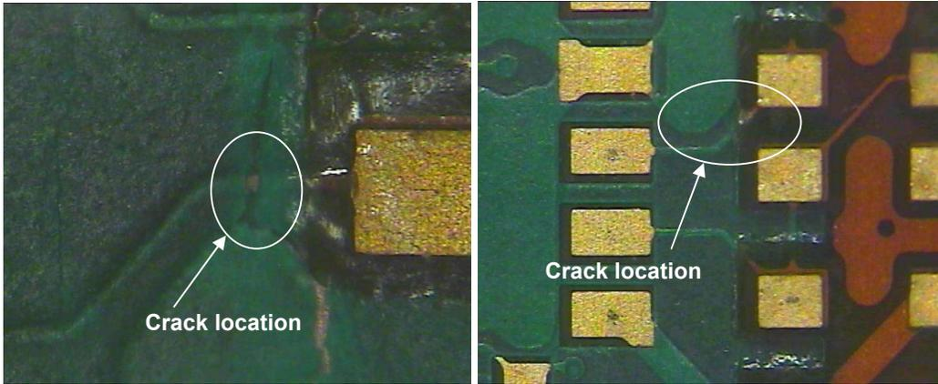
Figure.12: Soldermask cracking
