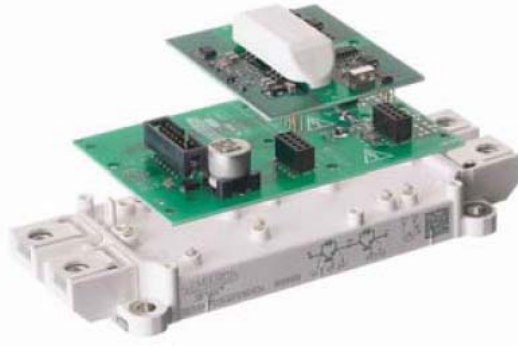
Figure D.1: SKYPER 32 PRO with adapter board on top of SEMiX module.
