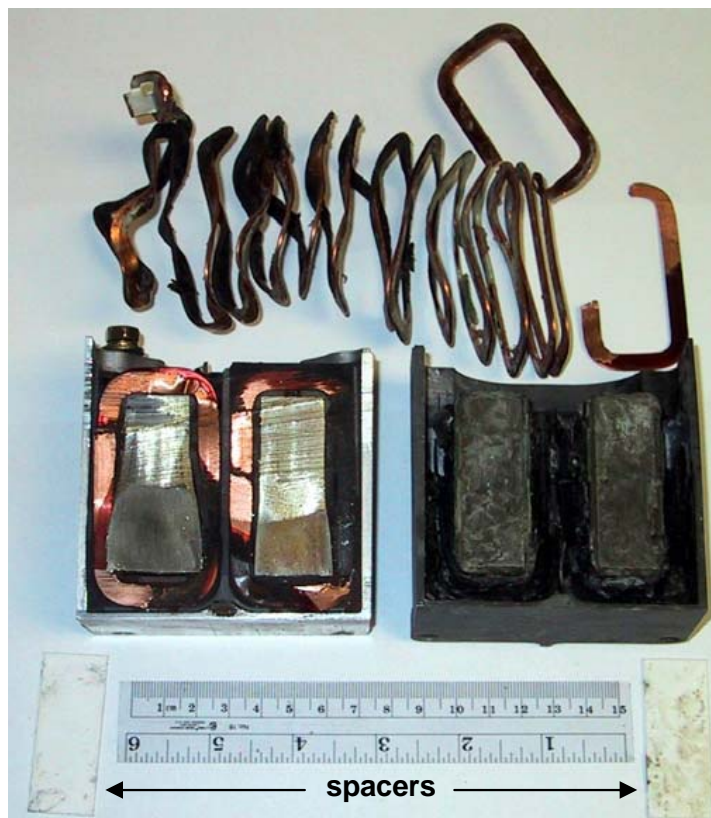
Figure 5.4: Picture of Prius THSII boost inductor with ceramic spacers.
