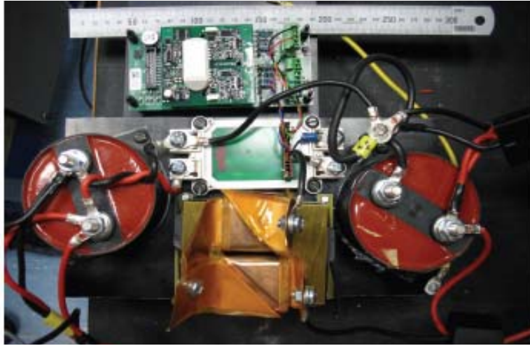
Figure 3.3: 2.5 kW, 125-250 V hard switched dc-dc converter setup.
