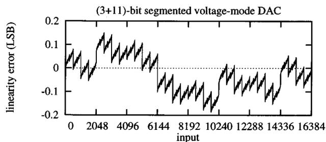
Fig. 6. Endpoint-corrected linearity error associated with the (3+11)-bit segmented voltage-mode DAC in Table III. The linearity error is given by  $(16383/V_{OUT}(16383))V_{OUT}(U) - U$ ,  $U = 0, 1, 2, \dots, 16383$ .
