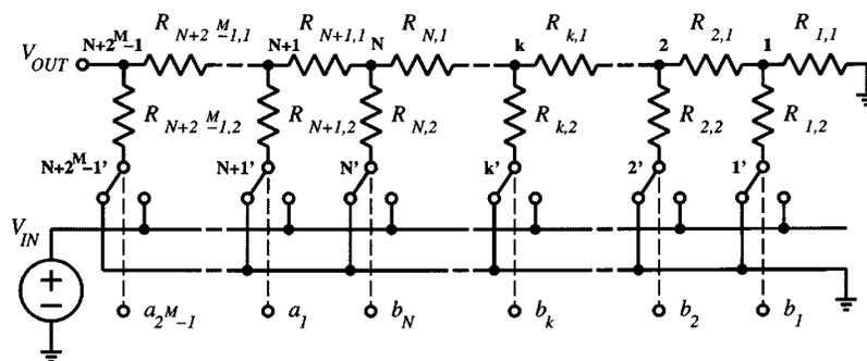
Fig. 5. Segmented voltage-mode resistive ladder DAC. In the nominal ladder,  $R_{k,2} = 2R$  for all  $k$ ,  $R_{1,1} = 2R$ ,  $R_{k,1} = R$  for  $k = 2, 3, \dots, N+1$ , and  $R_{k,1} = 0$  for  $k = N+2, \dots, N+2^M-1$ .
