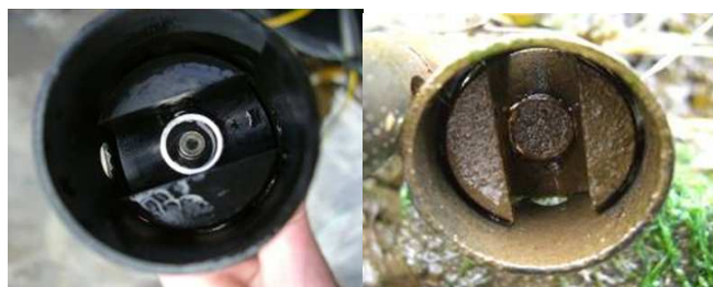
Figure 4: Photographs of a fouled (top) turbidity sensor and (below) after cleaning the same sensor.
