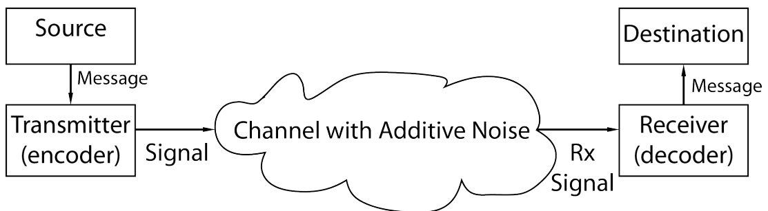
Figure 2.9: Block diagram of a generic communication system
