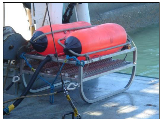
Figure C-4 Geo-Spark 1500 power supply and towed Geo-Source 400 Sparker source.
