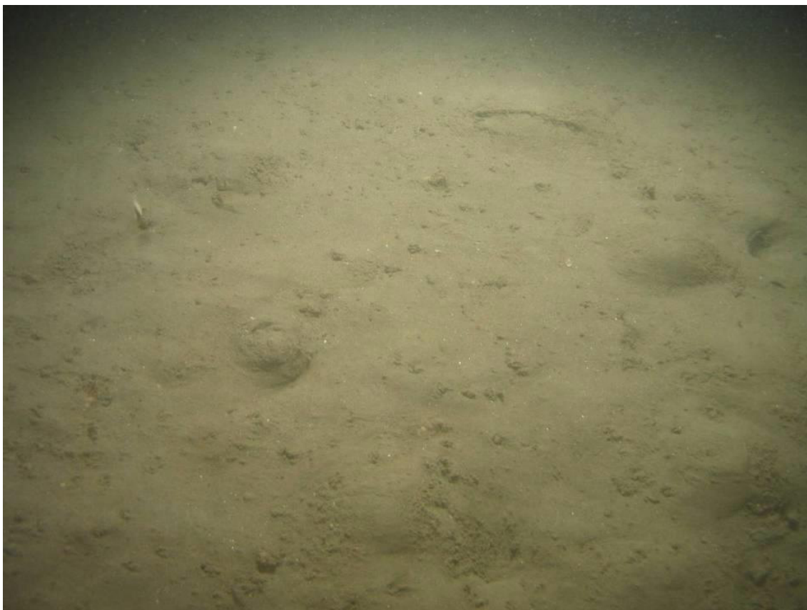
Figure B-25. Typical seabed image showing bioturbated muddy sands. Scale of view approximately 50 cm across.
