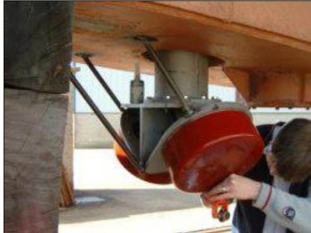
Figure C-3 Hull mounted multibeam transducer on the RVCeltic Voyager (photo of the Marine Institute).
