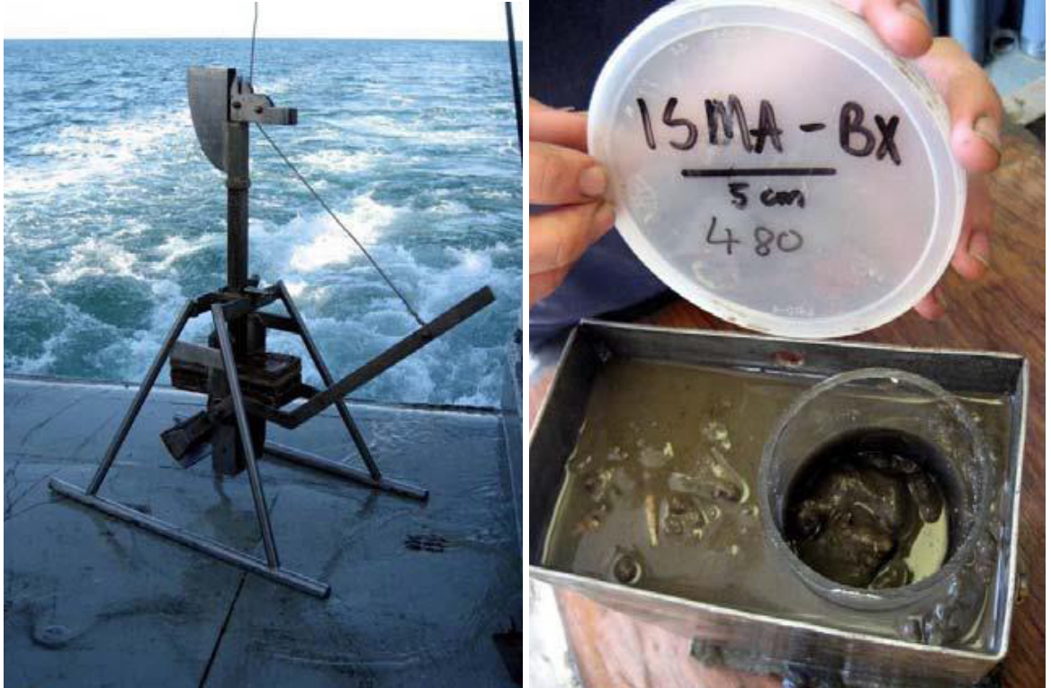
Figure B-8. The Reineck box-corer and retrieved sample showing the push-core inserted.
