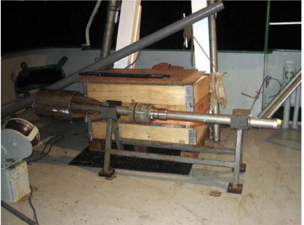
Figure B-9. Gravity corer with 1 m core barrel.
