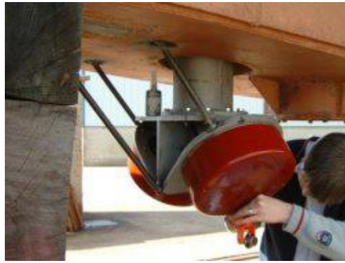
Figure B-3. Hull mounted multibeam transducer on the RV Celtic Voyager (photo of the Marine Institute).
