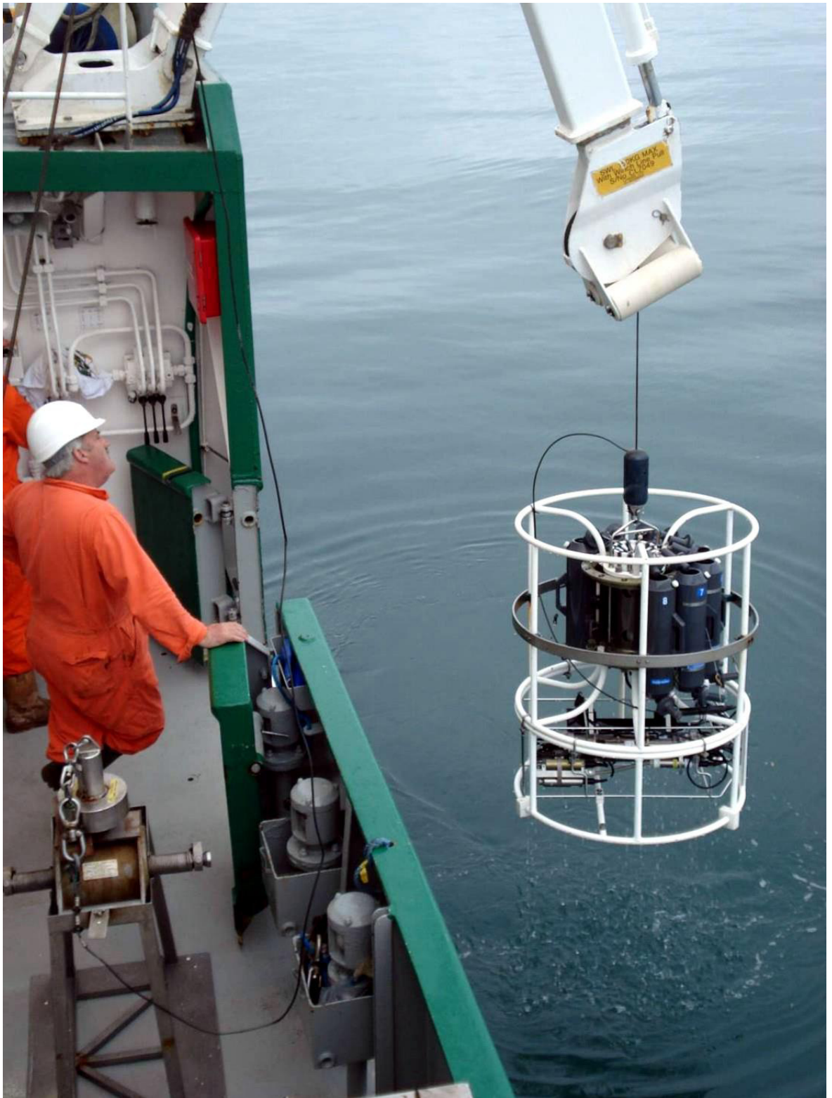
Figure B-5. Sea-Bird SBE 9plus CTD profiler being deployed
