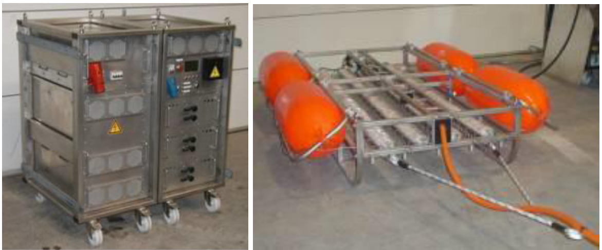
Figure B-4. Geo-Spark 6 kJ pulsed power supply and towed Geo-Source 400 Sparker source.
