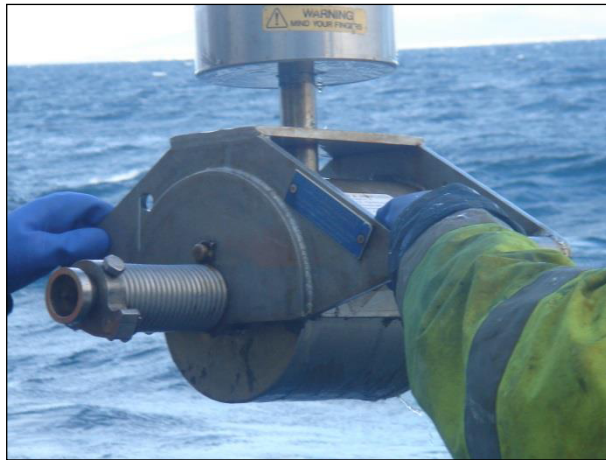
Figure C-6. Shipek sampler recovered after a successful deployment.
