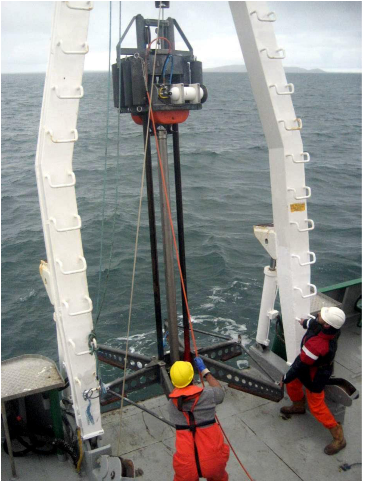
Figure B-10. The Geo-resources 6000 vibrocore being deployed.
