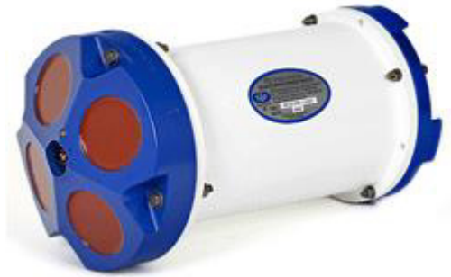
Figure B-6. The TRDI 600 kHz Workhorse Sentinel ADCP
