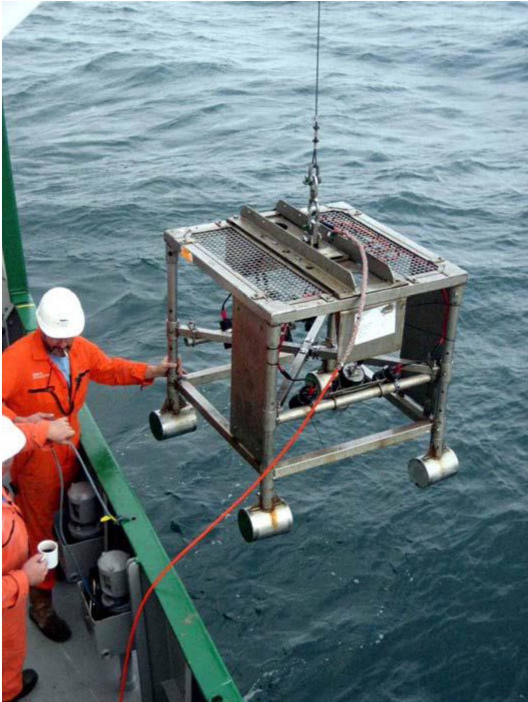
Figure B-11. The digital stills camera, flash and LED lamps housed in the camera frame being deployed off the starboard winch during the survey.
