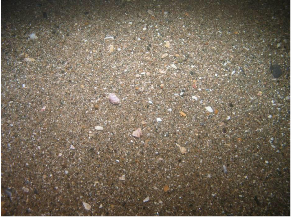
Figure B-44. Typical seabed image showing sorted coarse sands and shell hash from the sediment wave area. Scale of view approximately 50 cm across.
