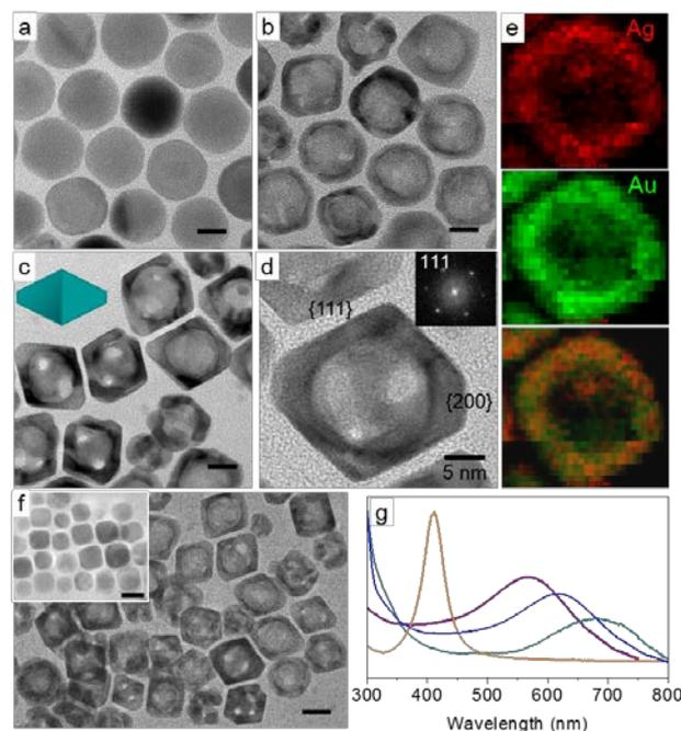
**Fig. 1** TEM image of (a) single crystal Ag NPs. After dropwise addition of (b) 0.25 ml and (c) 1 ml of AuCl<sub>3</sub>. Scale bar a-c is 10 nm. (d) HRTEM of hollow octahedral NP. (e) Elemental EDX mapping of octahedral NPs. (f) galvanic replacement of truncated cubic NPs. Inset: truncated cubic NPs. Scale bar is 10 nm. (g) UV-vis spectra of NPs showing red-shift in LSPR.
