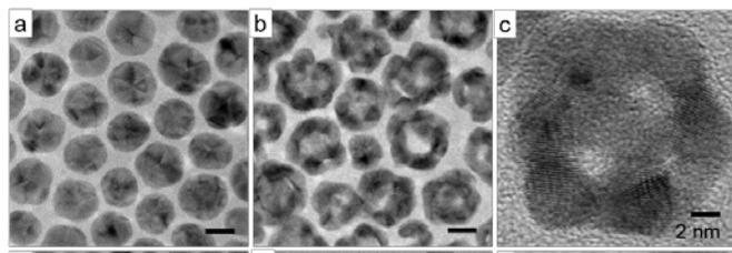
**Fig. 4.** (a) 15 nm (d) 8 nm (g) 6 nm MT Ag NPs and (b, e, h) after galvanic replacement with dropwise addition of 1 ml 0.2 mM AuCl<sub>3</sub> solution. HRTEM of AgAu (e) nanocage, (f) nanoring and (i) solid alloy NP.
