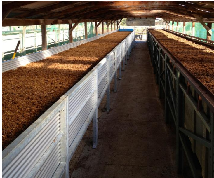
Figure 1.3 Flow-through vermicomposting beds (sonomavalleywormfarm.wordpress.com)
