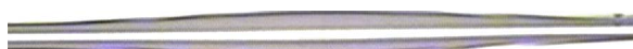
FIG. 6. Optical micrograph of a bottle resonator with a diameter of 12 \mu\text{m} and length of 300 \mu\text{m} . The bar is 10 \mu\text{m} .
