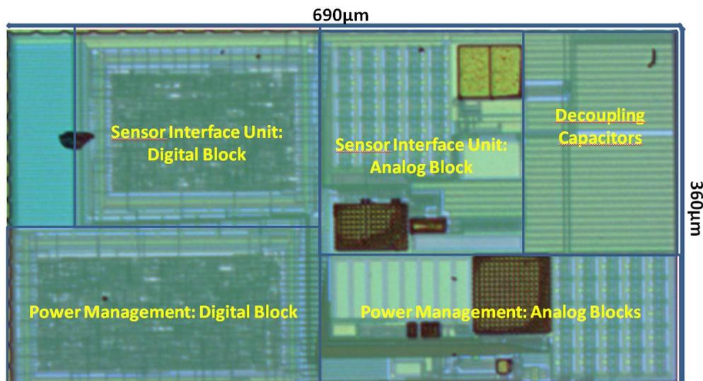
Figure 10. Chip microphotograph of the SiNAPS microsystem.
