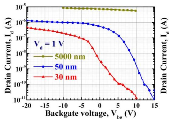
Figure 7.(A) SEM images of devices composed of a) 1, b) 3 and c) 20 Si NWs. In each case the wires are 1  $\mu$ m long and 20 nm wide. (B)  $I_d$ - $V_{bg}$  curves of devices composed of single SiNWs of length 1  $\mu$ m and widths of 30, 50, and 5000 nm.
