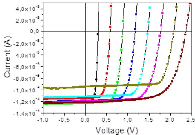
Figure 6. Simple minimodule with a total area of 7.8 mm<sup>2</sup> consisting of 8 nanowire solar cells connected in series by wire bonding (top) and I-V curves under AM1.5 illumination of cells 1 to 8 of the module connected in series.
