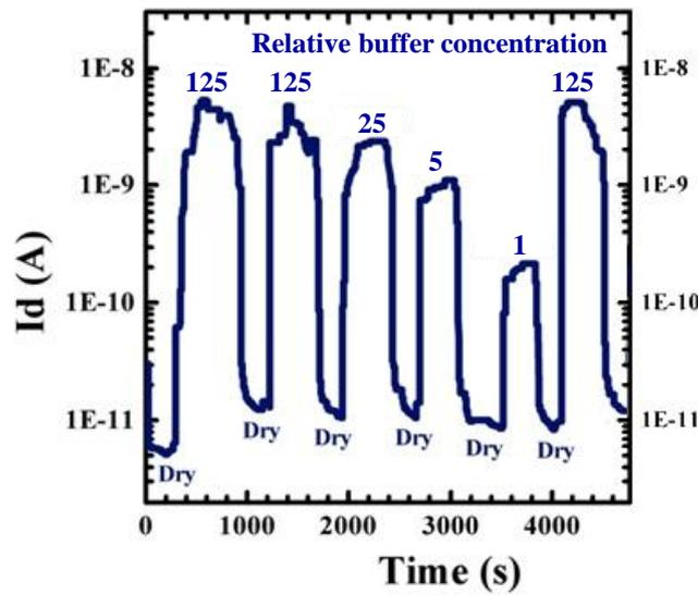
Figure 9. Time dependence of the drain current  $I_d$  whilst pH7 buffer solutions of various concentration are flown through the channel. Air was used to dry the channel in between administrations of buffer.
