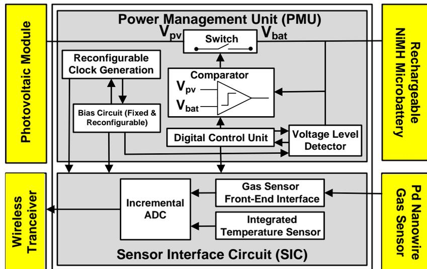
Figure 1. Block diagram of the SiNAPS electronic circuit.
