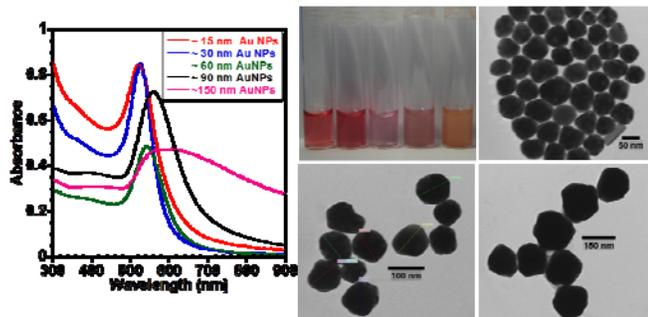
**Figure 1.** UV-visible spectra (left) of synthesized Au NPs. The corresponding colloidal solution (top left) and TEM micrographs of the Au NPs with diameter  $\sim 60$  nm (top right);  $\sim 95$  nm (bottom left) and  $\sim 150$  nm (bottom right).
