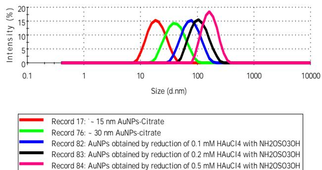
**Figure 2.** Size distribution by intensity obtained from DLS on synthesized Au NPs Au NPs with mean diameters of  $\sim 60$ ,  $\sim 95$  and  $\sim 150$  nm were obtained by reduction of  $\text{HAuCl}_4$  (0.1, 0.2 and 0.5  $\text{mmol L}^{-1}$  respectively) with HOS at room temperature ( $PDI < 0.17$ ).
