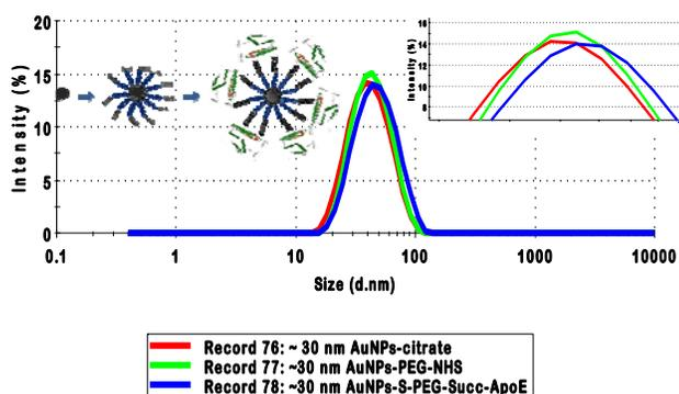
**Figure 3.** Size distribution by intensity obtained from DLS on 30 nm Au NPs-citrate before, and after PEGylation with NHS-PEG-S-S-PEG-NHS, and further attachment of ApoE protein through a biologically stable amide linkage; insert left (overall bioconjugation process Scheme 1 and 2), insert right show the Au NPs size increase after each step.
