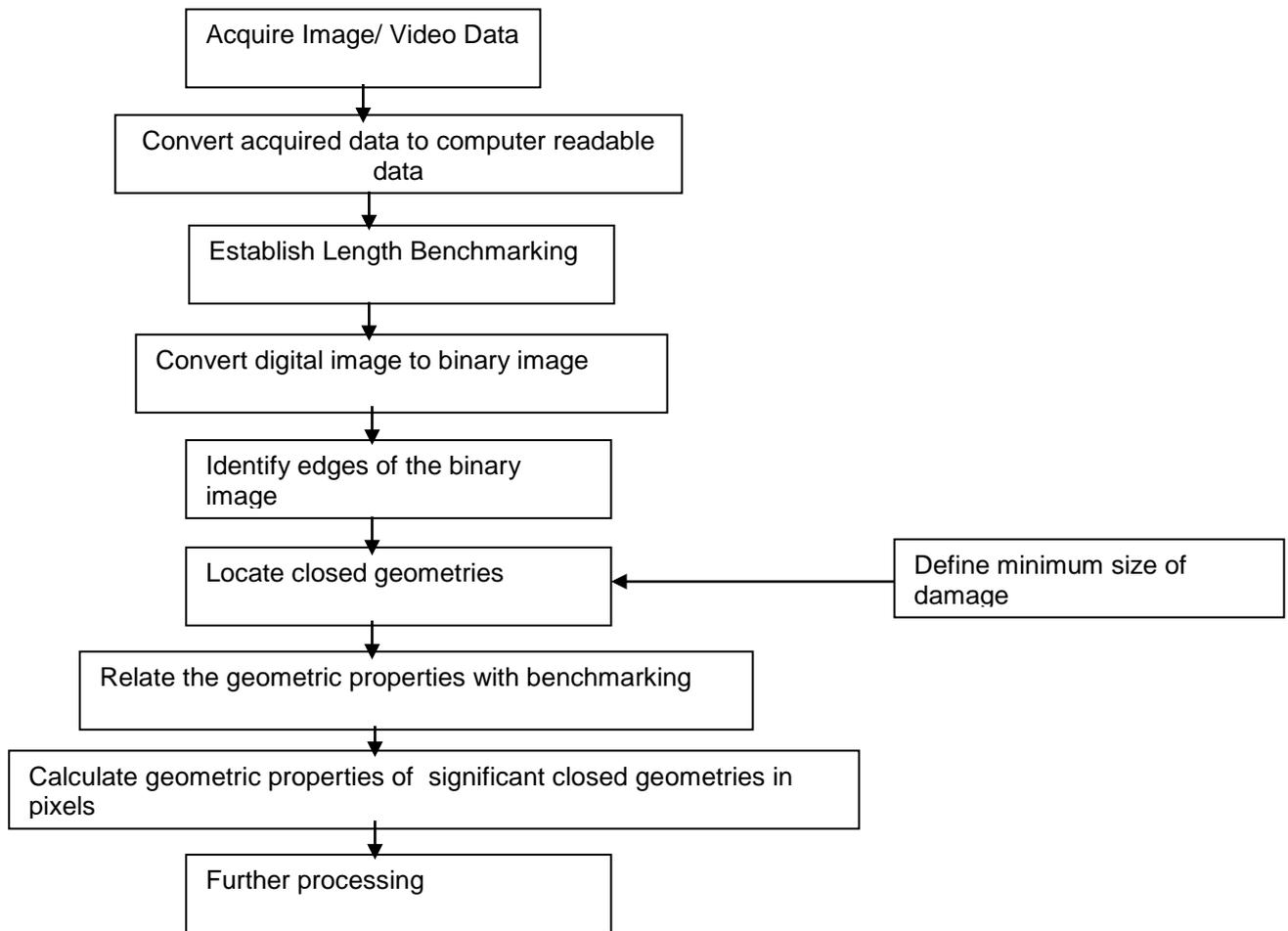
Figure 1. Schematic of Image Based Detection Scheme
