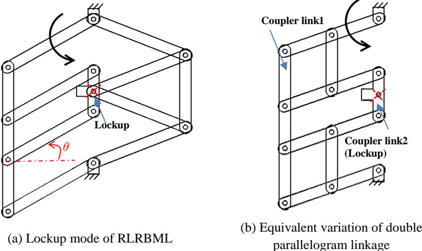
**Figure 4.** Lockup mode of the RLRBML
