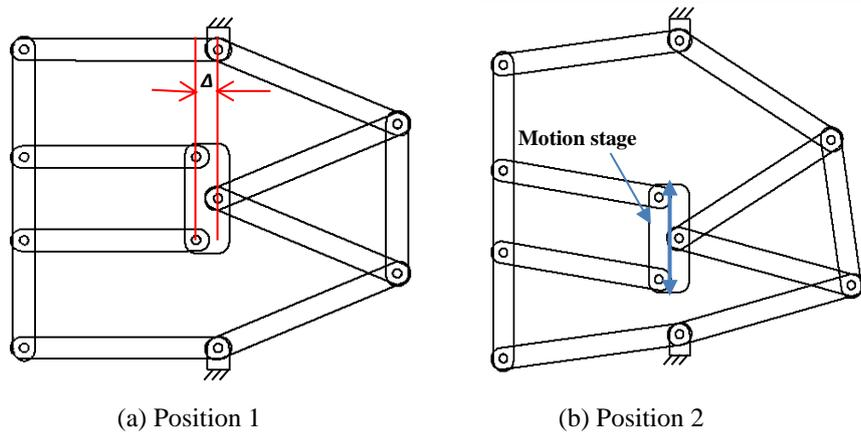
**Figure 8.** Single-mode linear rigid-body motion linkage 1
