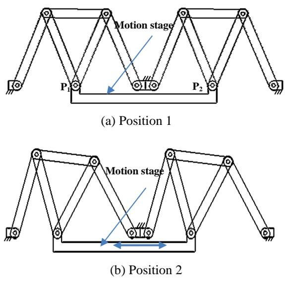
**Figure 9.** Single-mode linear rigid-body motion linkage 2
