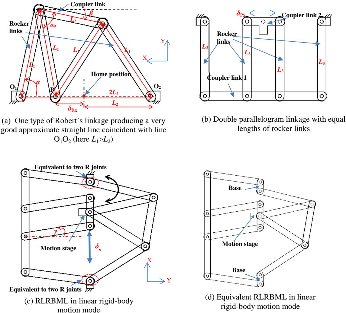
**Figure 1.** RLRBML and its two compositional units
