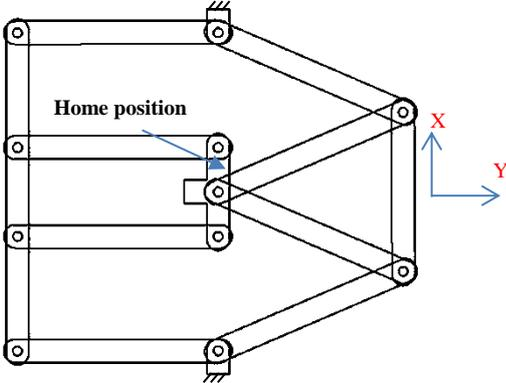
**Figure 3.** Singular configuration of the RLRBML
