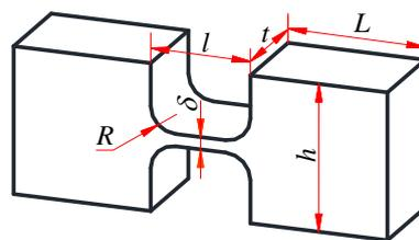
Fig. 2 Geometric parameters of corner-filletted flexure hinge
