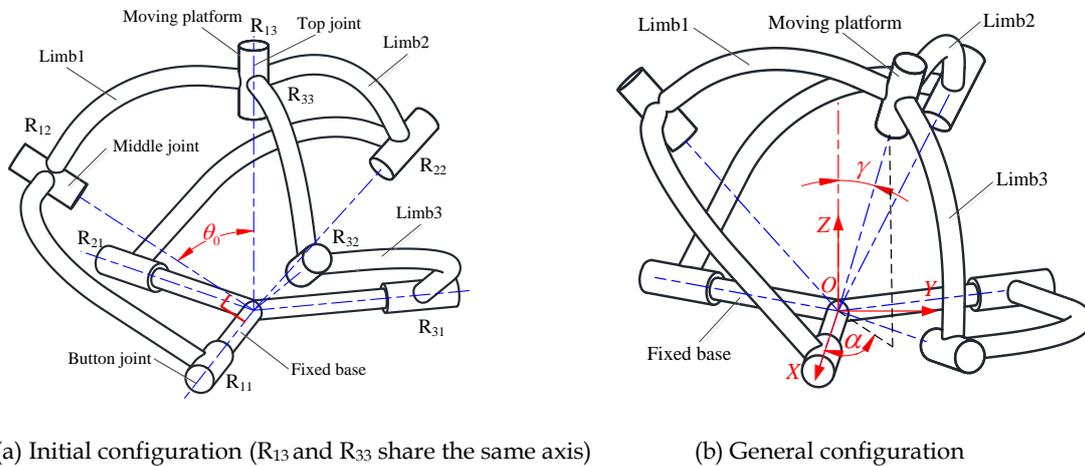
Fig. 1 Configuration of the 8R spherical rigid mechanism
