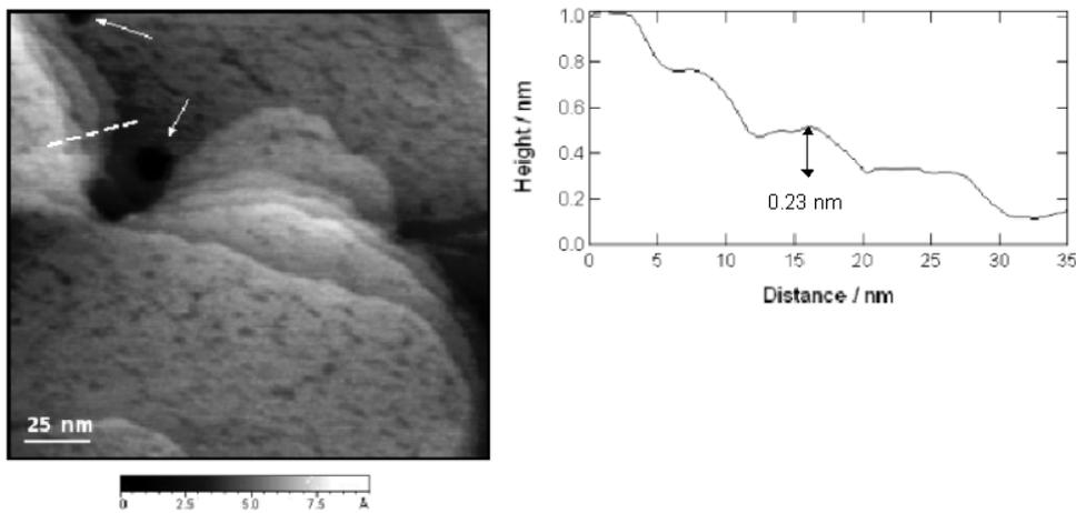
**Figure 7.** (a)  $200 \text{ nm} \times 200 \text{ nm}$  AFM image of the Au:1 surface shown in height-mapped grayscale. Examples of monatomic depressions in the Au surface are highlighted by arrows. (b) Height variation of successive monatomic Au step edges. This data represents the indicator line in the upper left of (a).
