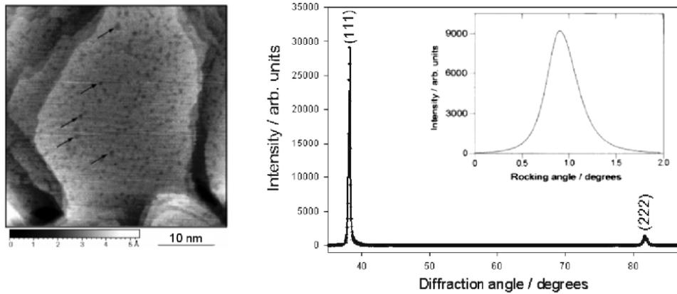
**Figure 3.** AFM image of the Au{111} surface showing the monatomic terraces. The corresponding GIXRD spectrum and rocking curves are also shown.
