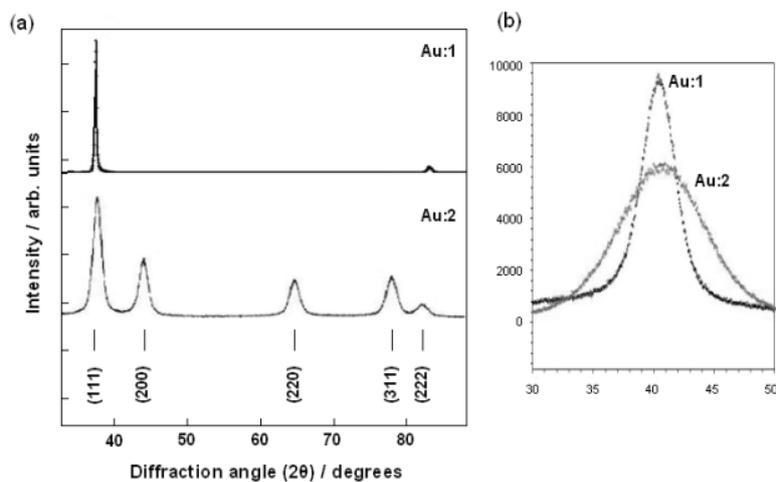
**Figure 6.** (a) GIXRD spectra of the Au:1 and Au:2 layers. On a logarithmic scale, no discernable peaks from 200, 220 or 311 reflections of the Au lattice could be observed for the Au:1 surface. (b) High resolution normalized GIXRD spectra of the Au:1 and Au:2 layers for the  $\{111\}$  peak.
