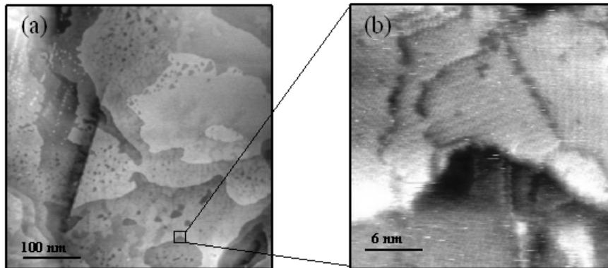
**Figure 4.** (a) 425 nm  $\times$  425 nm STM image of the SAM on Au{111} terraces. (b) 25 nm  $\times$  25 nm STM image of the area highlighted in (a) showing molecular scale domain boundaries and ordered alkanethiol molecule arrangement on Au{111} terraces.
