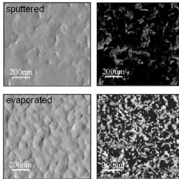
**Figure 8.** (a) AFM image of the SAM covered Au:1 surface (left panel), and its corresponding phase image (right panel). (b) AFM image (left panel) and corresponding phase image (right panel) for the Au:2 surface covered with the SAM.
