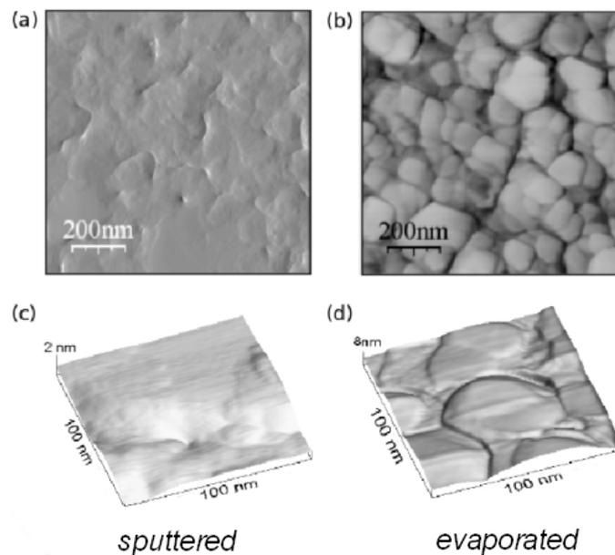
**Figure 5.** 1  $\mu\text{m}$   $\times$  1  $\mu\text{m}$  AFM image of (a) the Au:1 surface and (b) the Au:2 surface. (c) 100 nm  $\times$  100 nm higher magnification images of the smooth Au:1 surface and (d) the rougher Au:2 surface where multiple grains can be seen.
