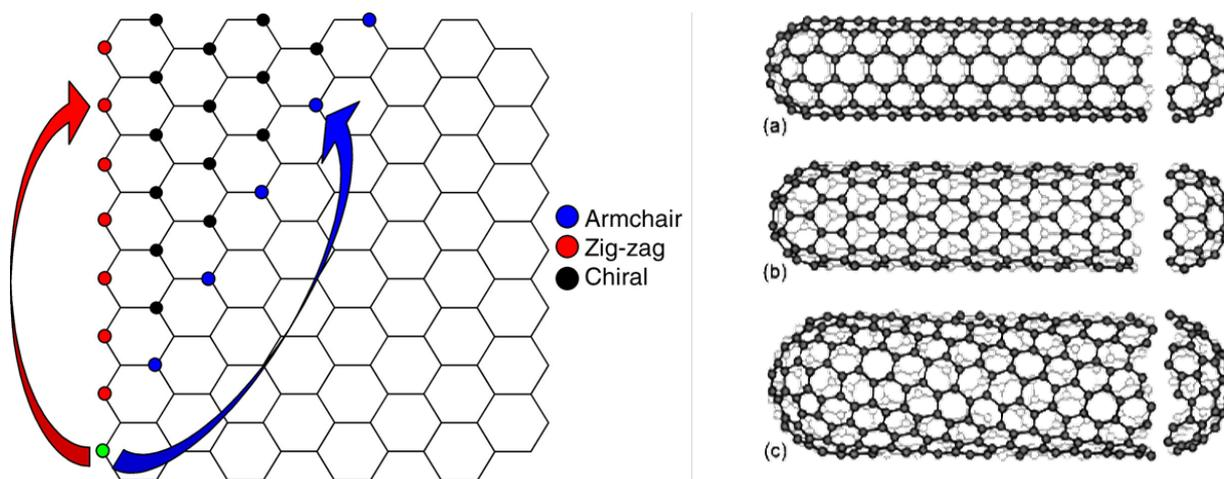
**Figure 3.** Graphic showing how a graphene sheet can be rolled to form different SWNT structures: (a) a metallic ‘zig-zag’ nanotube, (b) a metallic ‘armchair’ nanotube and (c) a chiral ‘semiconducting’ nanotube [3].
