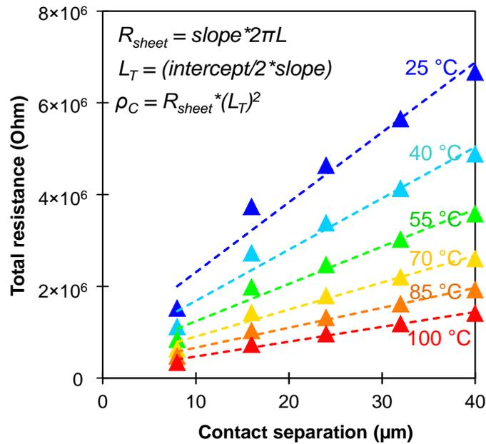
**Fig. 6 : Linearised total resistance versus contact spacing as a function of temperature, which is used to extract sheet resistance and MoS<sub>2</sub> resistivity. The Mo thickness was 10 nm prior to TAC.**
