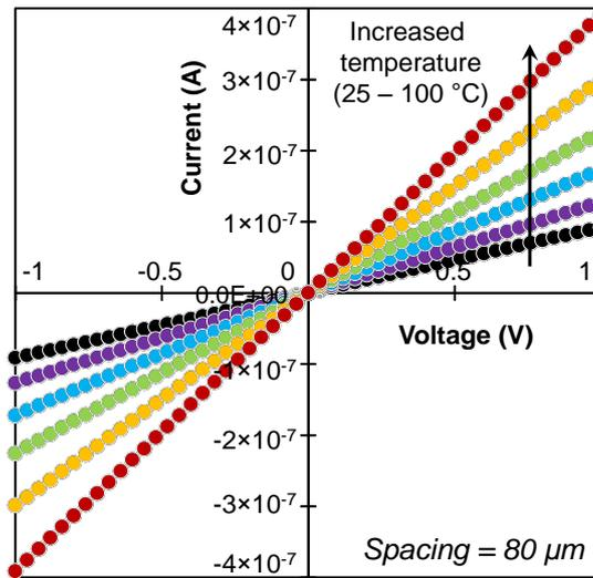
**Fig. 4 :** Measured current versus voltage characteristic in the MoS<sub>2</sub> circular TLM structure for different temperatures. The Mo thickness was 10 nm prior to TAC. The temperature dependence is consistent with a semiconductor behaviour.
