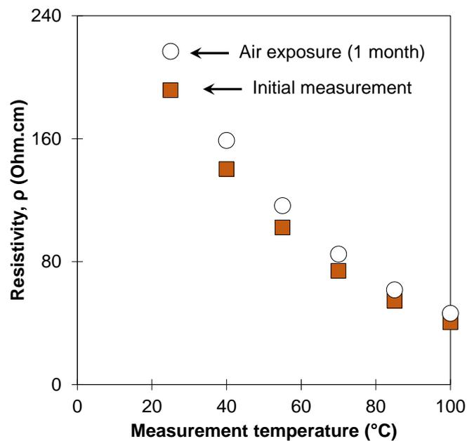
**Fig. 7 : Resistivity ( $\rho$ ) changes with air exposure. Orange points correspond to the initial measurements while the white points correspond to after 1 month of air exposure. At 25 °C there is a 13 % increase due to 1 month air exposure.**
