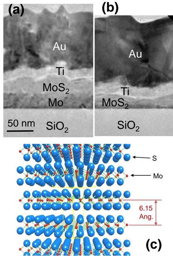
**Fig. 2 :** (a) Representative image of 30 nm Mo after TAC, forming MoS<sub>2</sub> laying on top of unreacted Mo. (b) Representative image of 10 nm Mo after TAC, completely converted to MoS<sub>2</sub>. (c) A schematic shows the lattice spacing in MoS<sub>2</sub>. The lattice spacing of 6.15 Angstrom allows us to identify the regions of MoS<sub>2</sub>.
