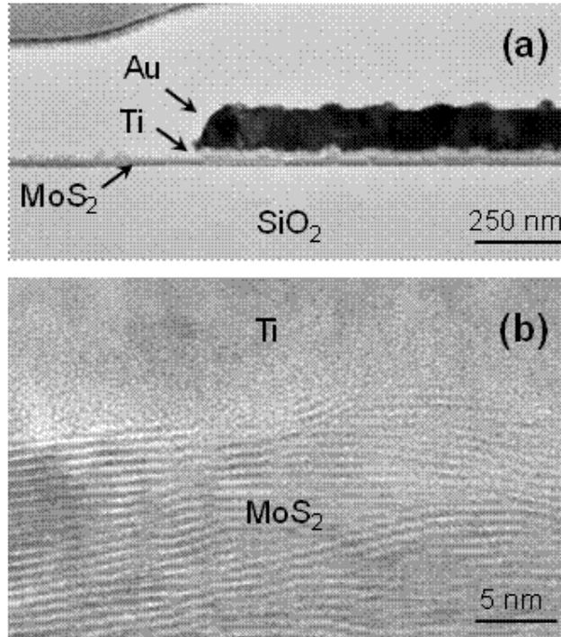
**Fig. 1 : Representative images of the 10 nm Mo after TAC, forming approximately 20 nm of MoS<sub>2</sub>. (a) A wide view of MoS<sub>2</sub> on a SiO<sub>2</sub>/Si substrate. On the right-hand side the Ti/Au metal contact is visible. The MoS<sub>2</sub> layer is continuous across the surface. (b) The layered structure of MoS<sub>2</sub> is visible in the higher resolution image.**
