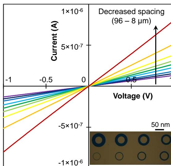
**Fig. 3 : Representative measured current versus voltage characteristic in the MoS<sub>2</sub> circular TLM structure as a function of contact spacing. The Mo thickness was 10 nm prior to TAC. The current is linear with respect to voltage and passes through the origin. The current increases with decreased contact spacing as expected. The inset shows an optical image of the circular TLM structure.**
