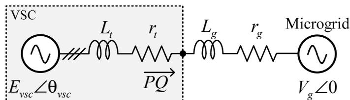
Fig. 1. Equivalent circuit of a three-phase grid-tied VSC
