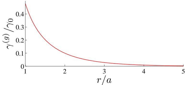
Figure 4: (Color online) Normalized spontaneous decay rate of a two-level atom into the fundamental guided mode,  $HE_{11}$ , as a function of distance between the atom and the axis of the optical nanofiber for a radius  $a = 200$  nm.
