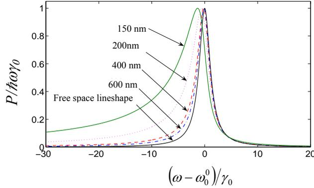
Figure 5: (Color online) Frequency dependence of the fluorescence power from a Rb cloud coupled into the optical nanofiber for a fiber radius  $a = 200$  nm and an atomic cloud radius  $R = 600$  nm (blue), 400 nm (red), 200 nm (purple), and 150 nm (green). The solid black line shows the free space lineshape and all lines are normalized to a maximum value of 1 for ease of comparison.
