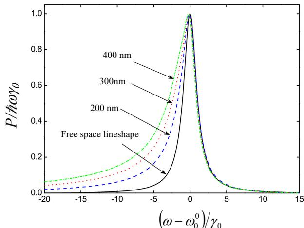
Figure 7: (Color online) Frequency dependence of the fluorescence power from a Cs cloud coupled into the optical nanofiber for redshift contributions from both the van der Waals and Casimir-Polder effects. The cloud radius is  $R = 400$  nm and the nanofiber radius is varied. The solid black line shows the free space lineshape and all lines are normalized to a maximum value of 1 for ease of comparison.
