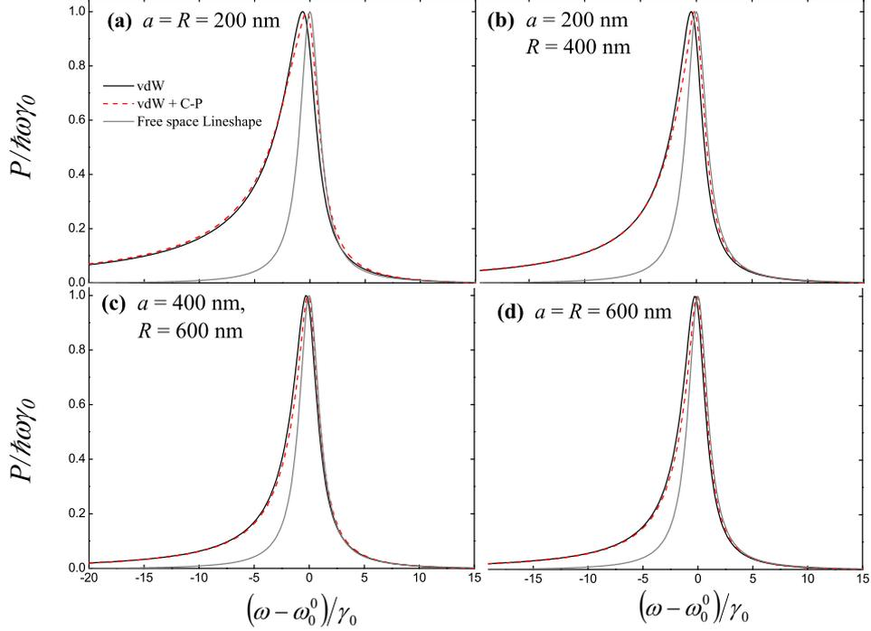
Figure 8: (Color online) Frequency dependence of the fluorescence power from a Cs cloud coupled into the optical nanofiber for different lineshape contributions: van der Waals effect only (black), Casimir-Polder + van der Waals (red), for different cloud radii and fiber radii. All lines are normalized to a maximum value of 1 and the free space lineshape is provided for ease of comparison between the curves.
