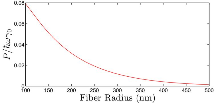
Figure 9: (Color online) Power coupled into a nanofiber as a function of fiber radius. The power shown is the maximum power for each value of fiber radius. The data was plotted for a Rb cloud with  $R = 500$  nm.
