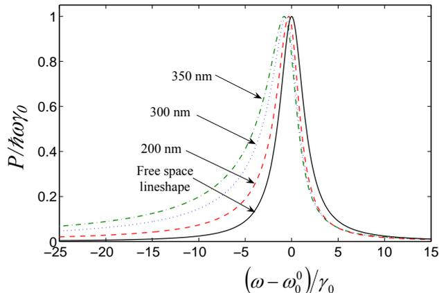
Figure 6: (Color online) Frequency dependence of the fluorescence power from a Cs cloud coupled into the optical nanofiber for a cloud radius  $R = 300$  nm and a nanofiber radius of 200 nm (red), 300 nm (blue), and 350 nm (green). The solid black line represents the free space lineshape. All lines are normalized to a maximum value of 1 for ease of comparison.
